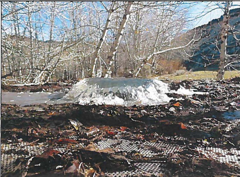
3-13-2014 Vertical flow from CDN's bubbler pipe. Estimated flow using vertical pipe equation at 1,372 gpm based on 3½ inches of rise over the 20-inch diameter pipe. Elk Pen flow-meter showed 700 gpm a few minutes later when E. Squires and C. Honsinger visited and read it.
