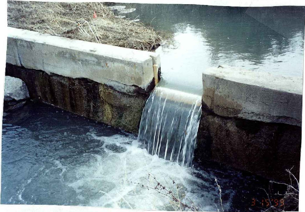
D/S measurement : H=0.38' L=2.0' From Tables, pg. 260, 1.56 cfs
