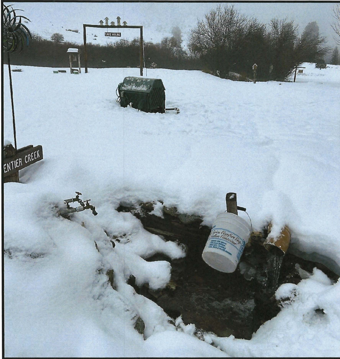
Photo 7- Step pool on the outlet from the pond. About 2' drop into the pool made bucket full measurements possible using the graduated bucket hanging on the post next to the 6" PVC pipeline. The green plastic pump house is visible in the left center of the image.
