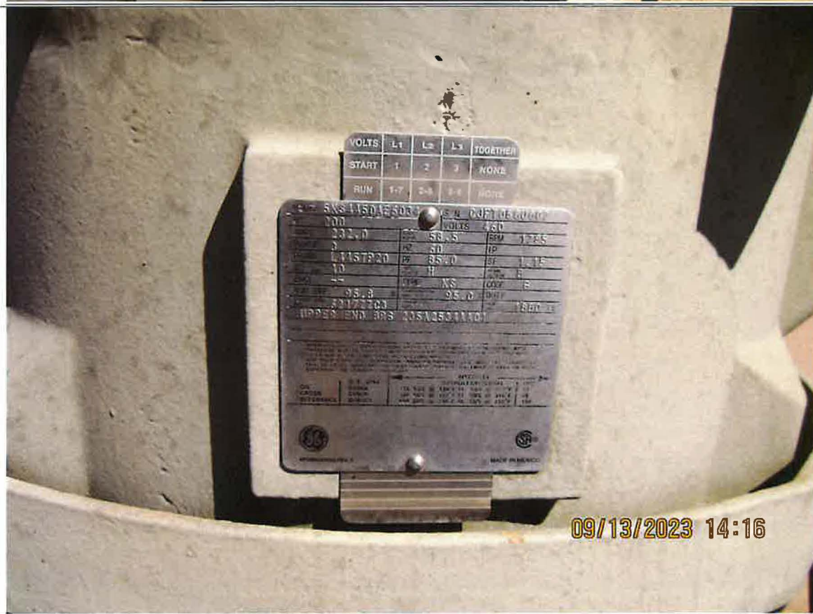
Figure 4. GE motor, model SK445DAE6034.
