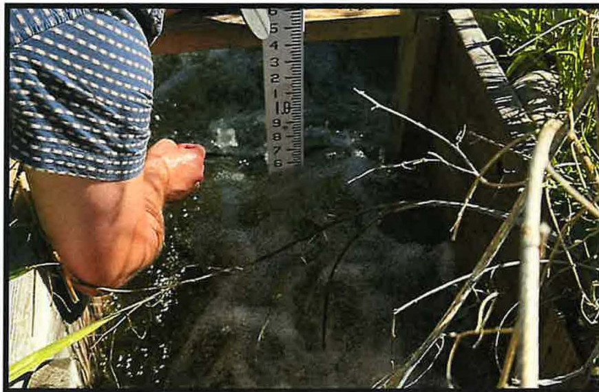
Photo 2- A discharge measurement made using a staff gauge. The bottom of the weir is flat. The structure and installation of the weir is not identifiable as any standard measuring device.
