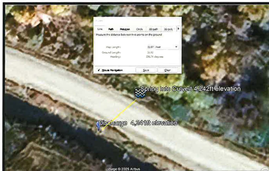
Figure 1- Google Earth Pro elevation (1ft drop) and length measurements (31.87ft) for corrugated steel culvert pipe passing under Lemhi Rd.
