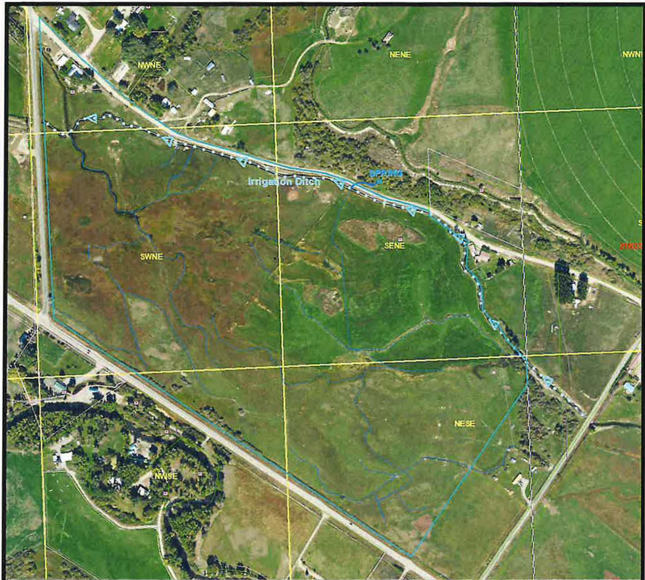
Figure 4- System Diagram- Spring water comingles with irrigation water in the irrigation ditch, then conveyed throughout the POU via lateral gravity fed ditches (darker blue lines).
