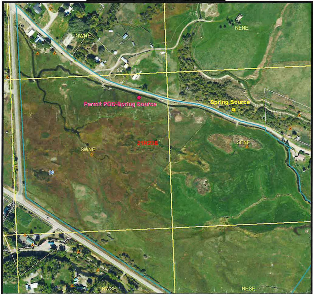
Figure 1- (GIS NAIP Imagery)- The permit place of use is outlined in blue. The permit spring-source point of diversion (POD) indicated by the purple point in the SWNE of section 30. The actual spring source POD indicated by the yellow point, is in the SENE of section 30. The proposed amendment will correct the legal description of the location of the spring source based on the GPS coordinates recorded during the field examination.
