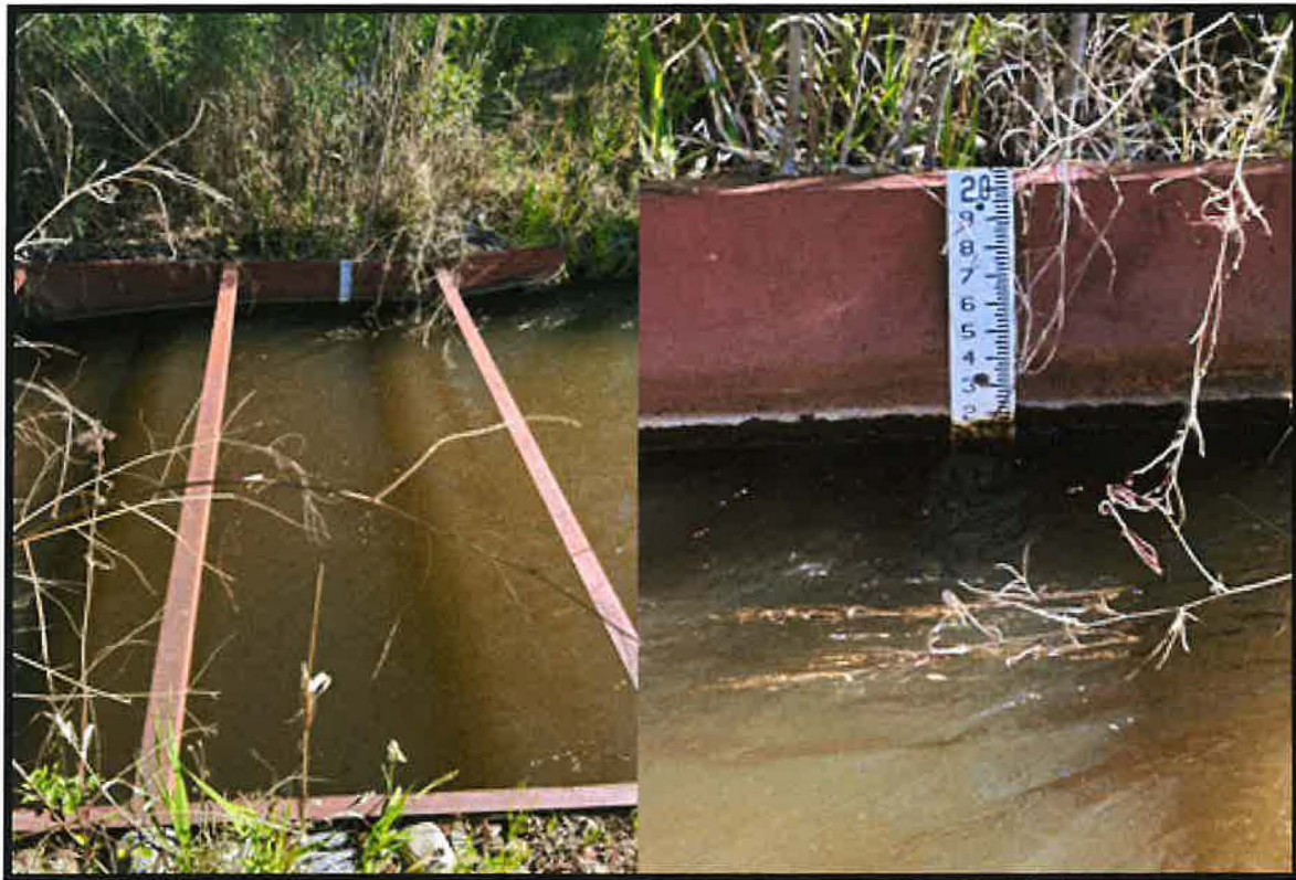
Photos 3 & 4 - Broad crested measuring weir just downstream of the headgate for the L-6. Reading observed at 1.14ft.
