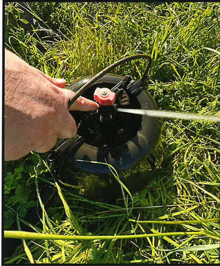
Photo 12 – Irripod with red tip at the end of the line. All 11 sprinklers have the same components.
