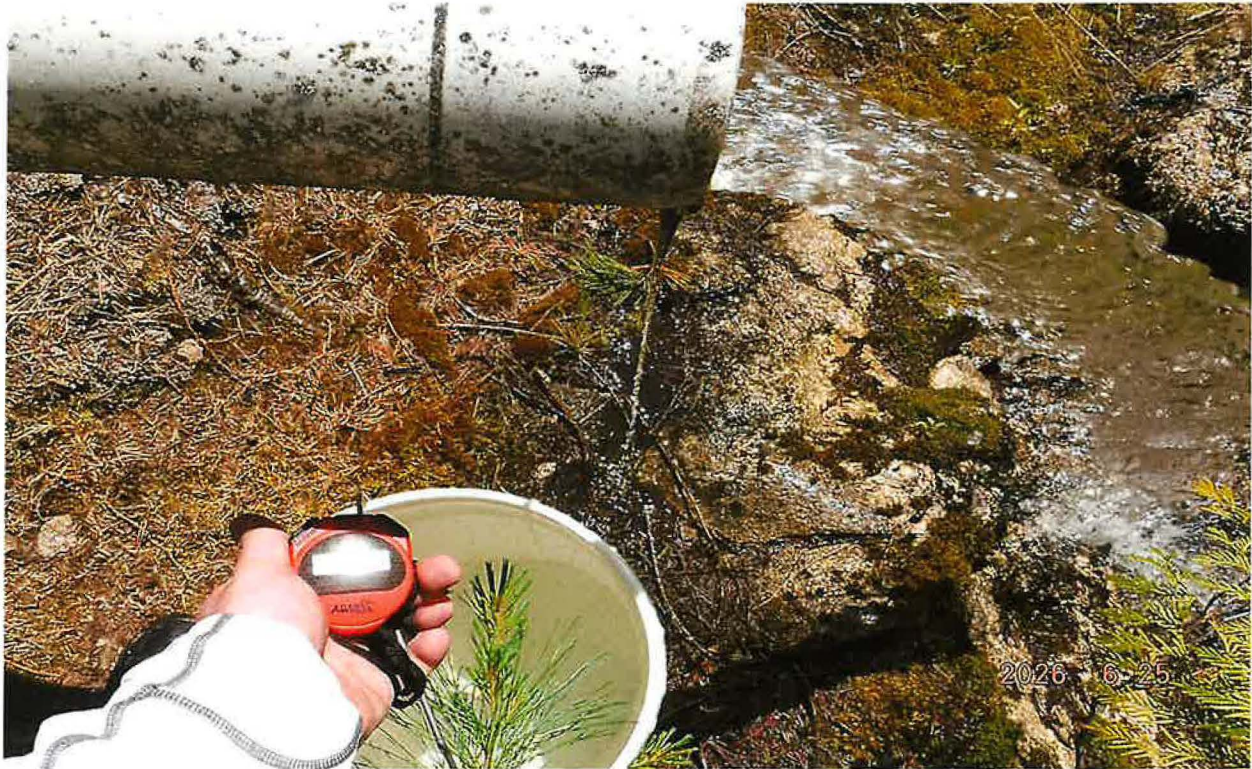
5-GAL BUCKET MEASUREMENTS TAKEN FROM OVERFLOW DISCHARGE PIPE AT FALL CREEK
