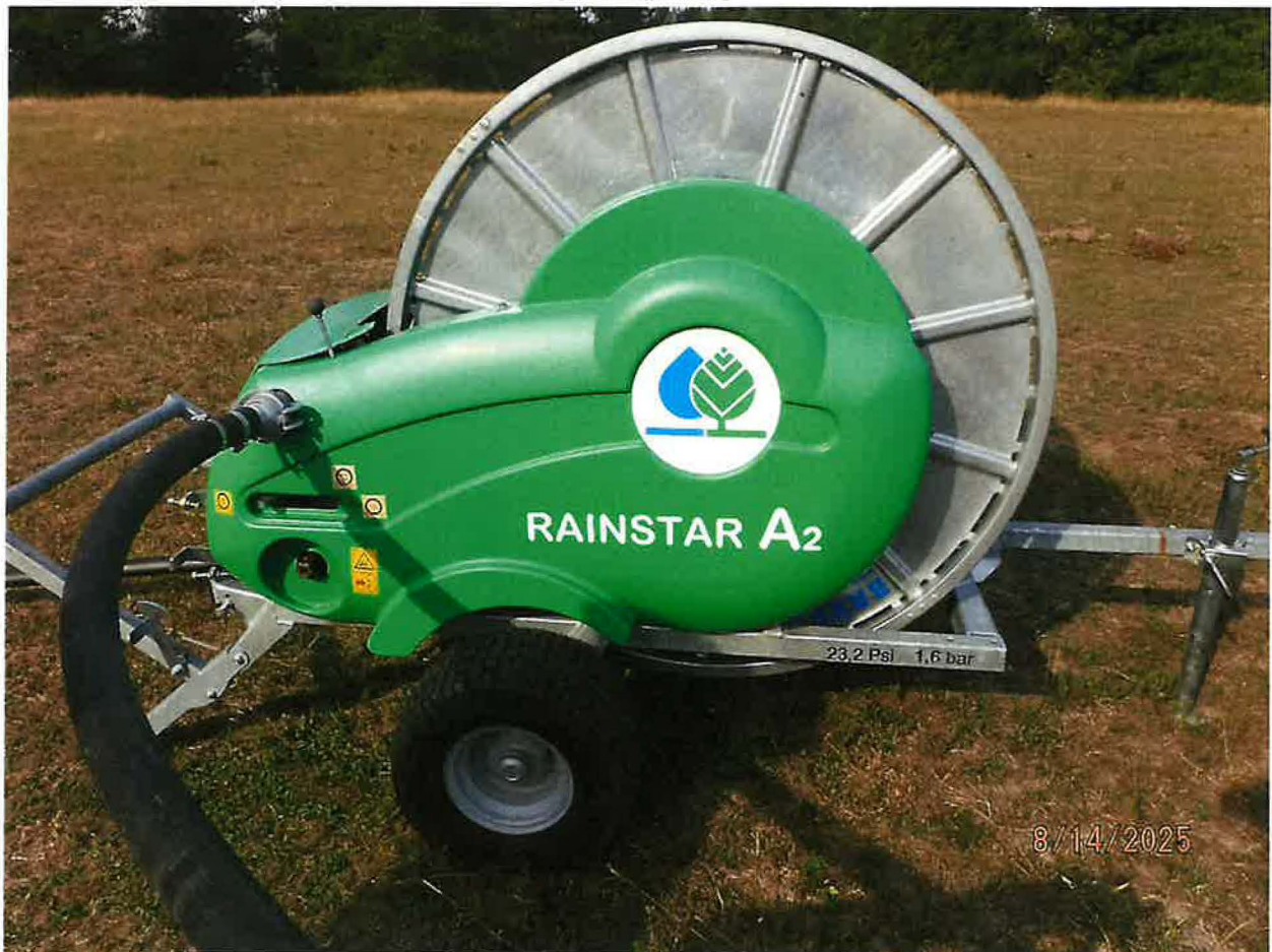
IRRIGATION POU – LAST IRRIGATION RISER PIPE CONNECTED TO BIG WHEEL SPRINKLER
