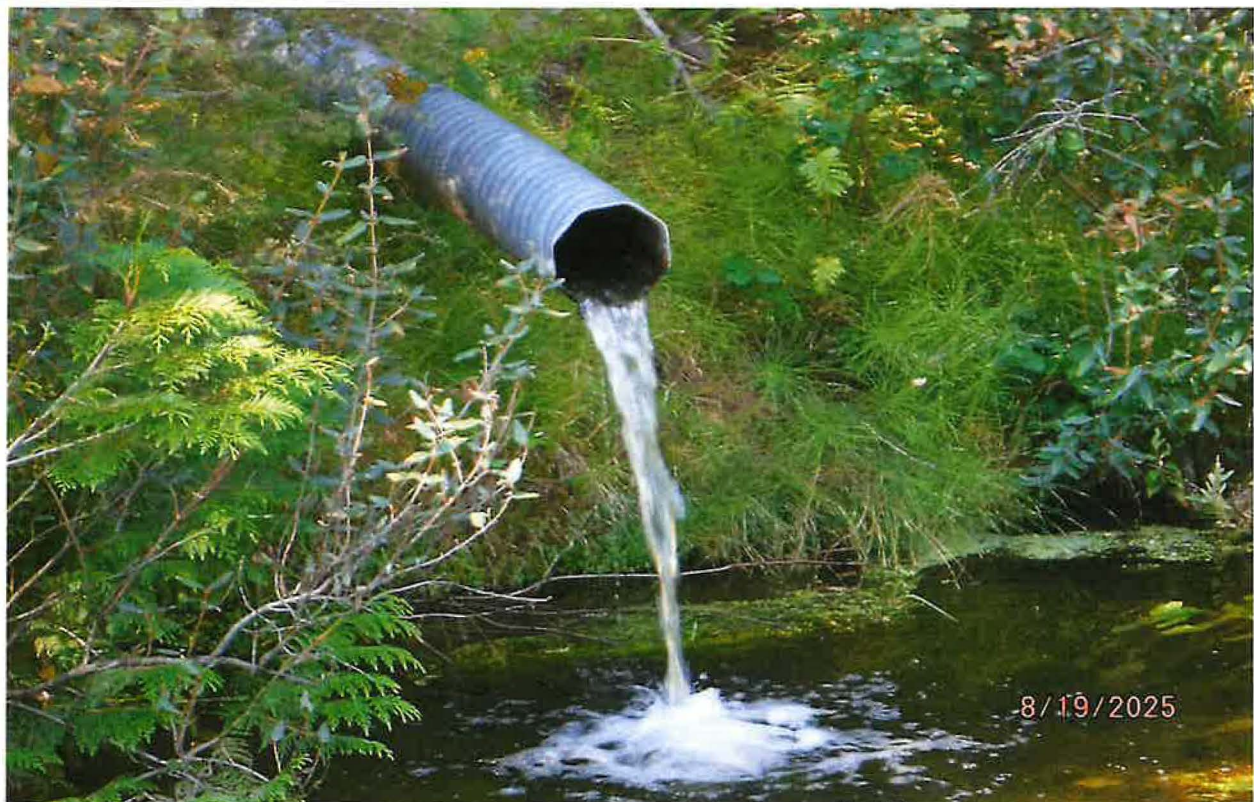
RECREATION POU – INFLOW FROM CONVEYANCE DITCH TO STORAGE POND #2 ; INFLOW 5-GAL BUCKET WAS MEASURED AT 13.55 SECONDS
