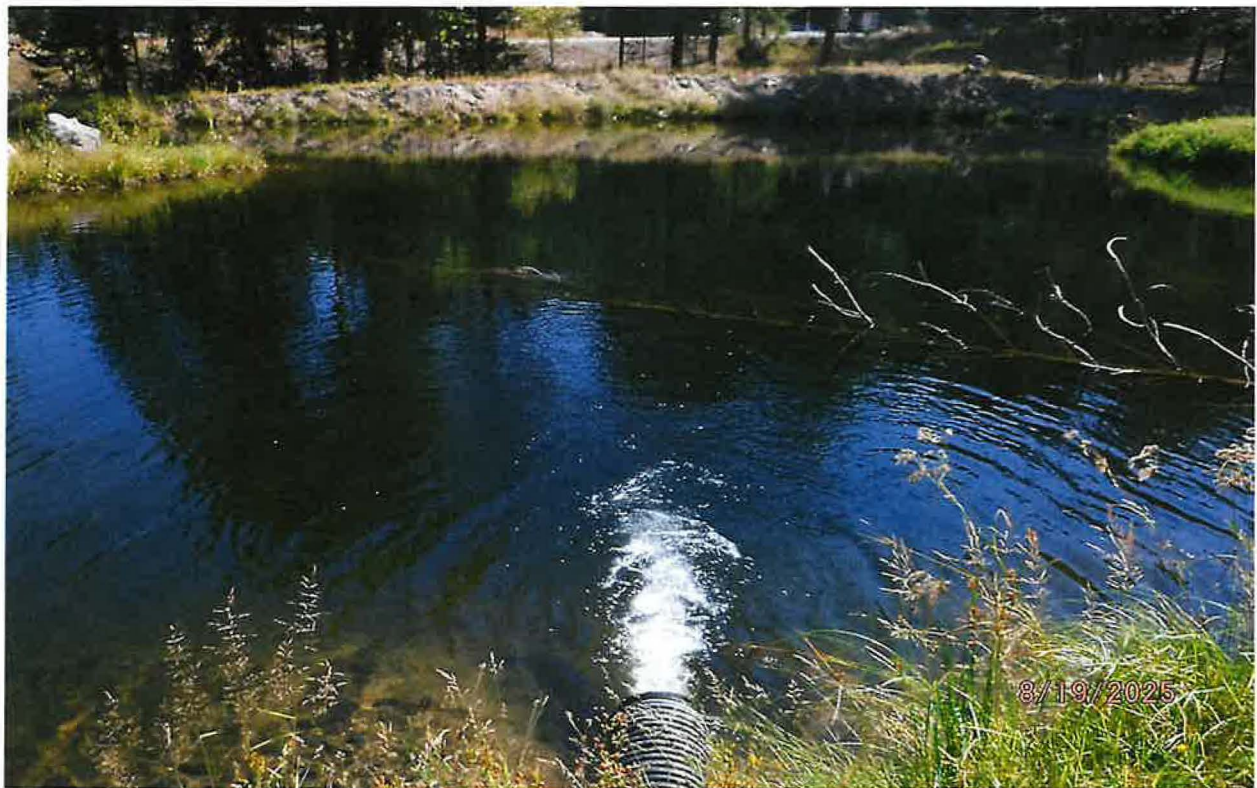
INFLOW 5-GAL BUCKET WAS MEASURED AT 2.94 SECONDS
