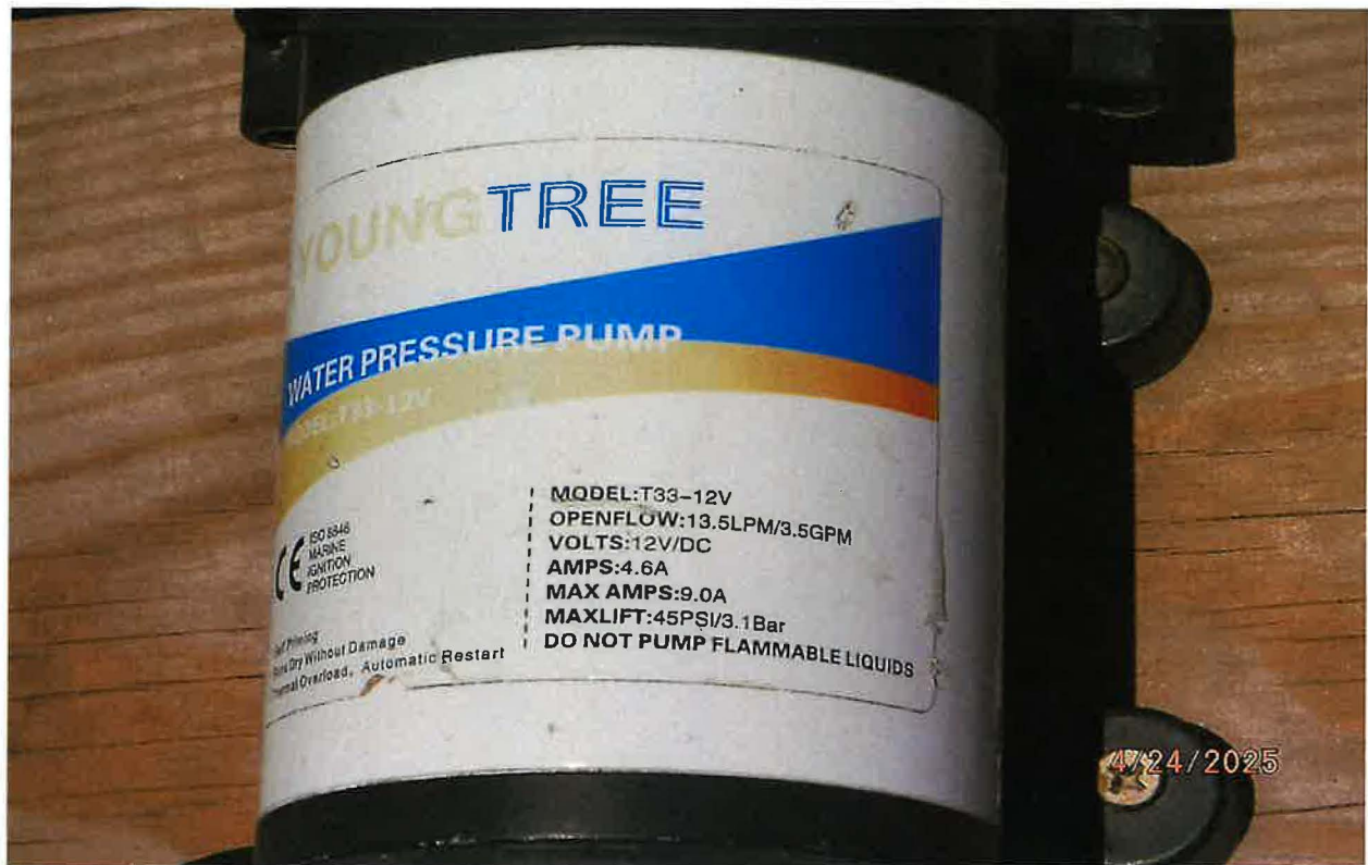
DIVERTING WORKS – 12V/DC 3.5 GPM PUMP ATTACHED TO 4-WHEELER TRAILER USED TO DIVERT UNNAMED STREAM WATER FROM COLLECTION POOLS
