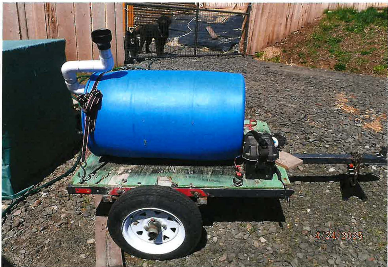
PORTABLE COLLECTION TANK USED TO TRANSFER STREAM WATER TO STORAGE TANK(S)
