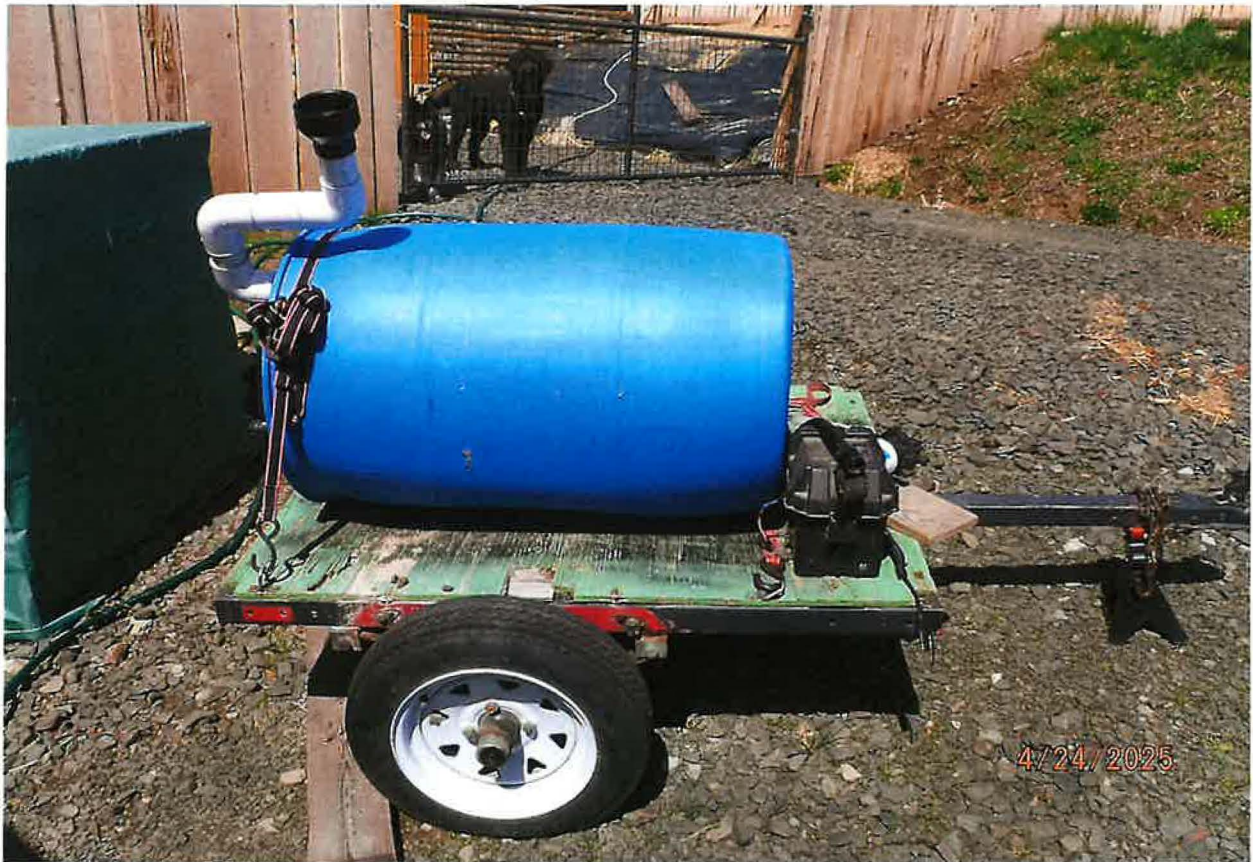
PORTABLE COLLECTION TANK USED TO TRANSFER STREAM WATER TO STORAGE TANK(S)
