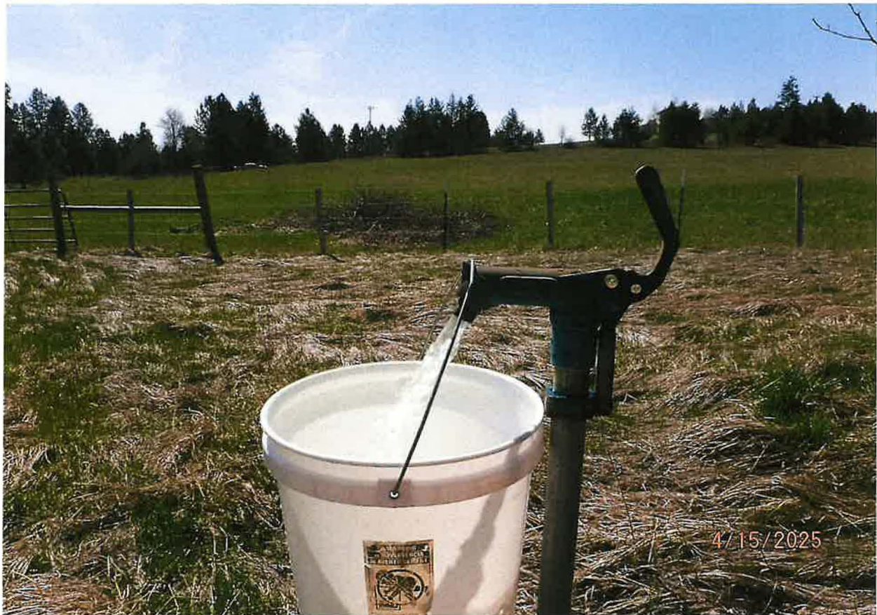
5-GAL BUCKET MEASUREMENT (3EA) TAKEN FROM HYDRANT LOCATED 10 FT OUTSIDE SPRING CISTERN WITH PUMP.
