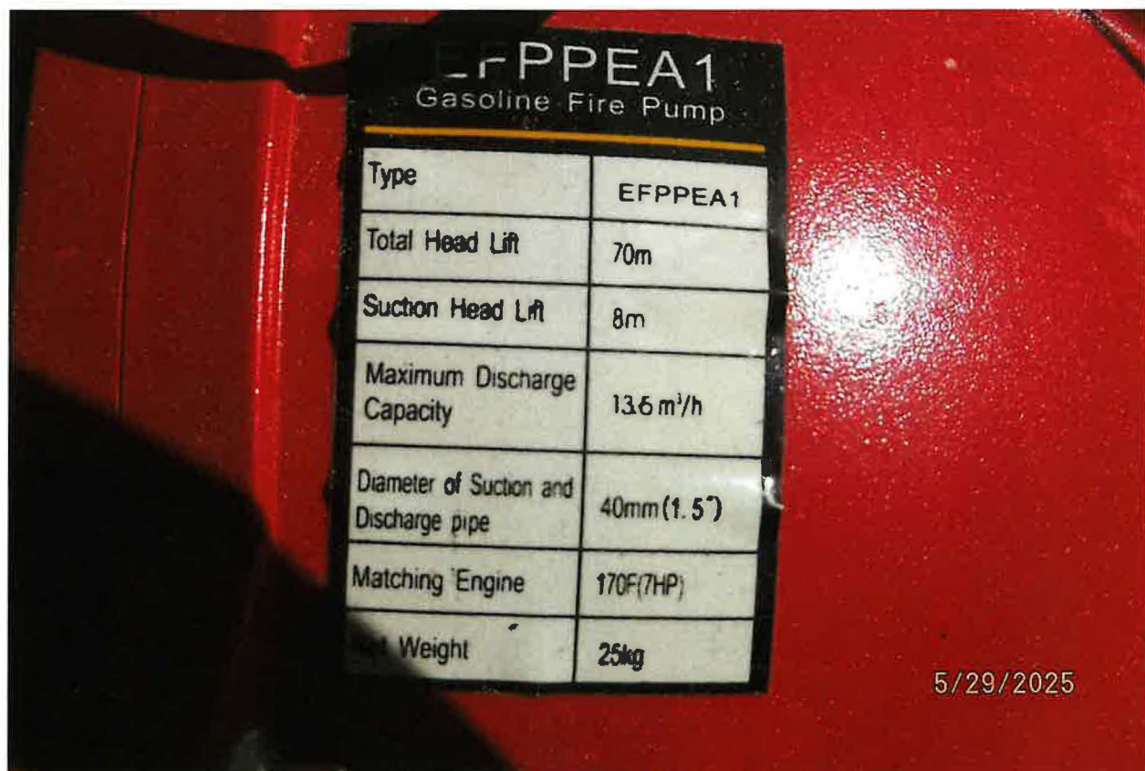
POD – DIVERTING WORKS 1.5-INCH SUCTION/DISCHARGE FIRE PUMP TYPE EFPPEA1. WATER CONVEYED BY 1.5-INCH FIRE HOSE 450FT TO POND
