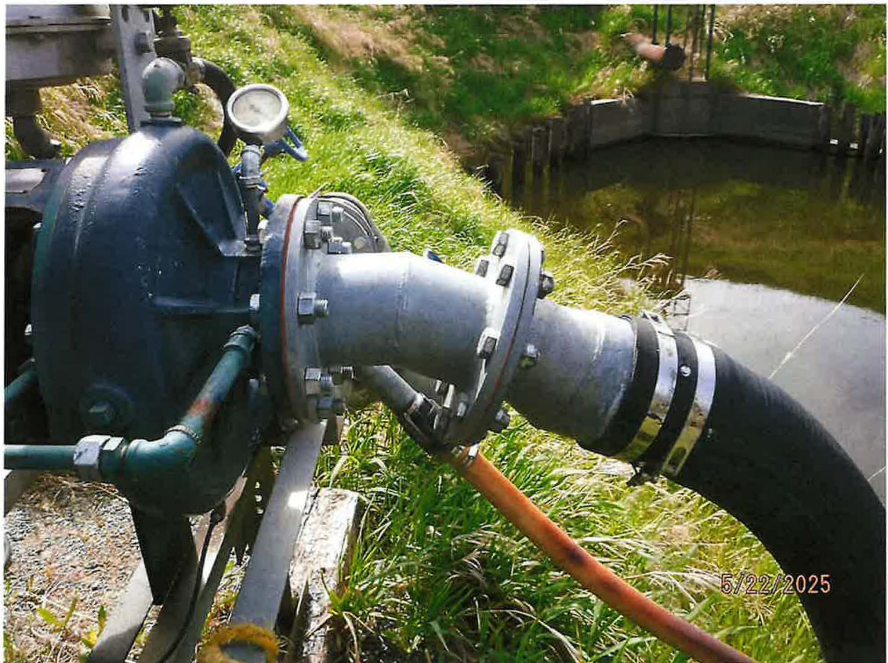
DIVERTING WORKS – FLEXIBLE 6-INCH INTAKE HOSE WITH SCREEN ATTACHED TO CORNELL CENTRIFUGAL PUMP SUCTION FLANGE
