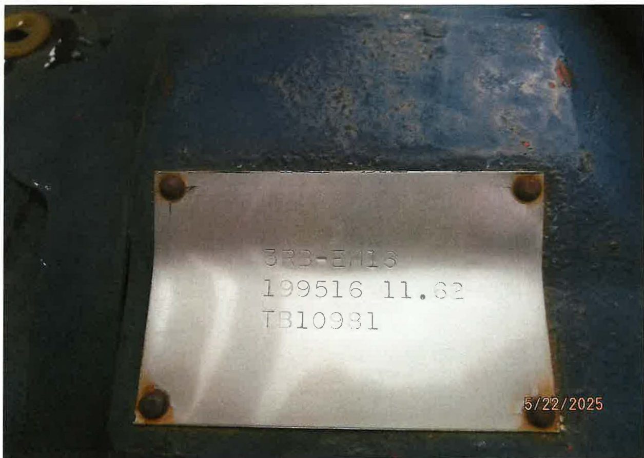
POD – DIVERTING WORKS INCORPORATE A CORNELL BRAND CENTRIFUGAL PUMP MODEL NO. 3RB-EM16, DIESEL FUEL POWERED PUMP
