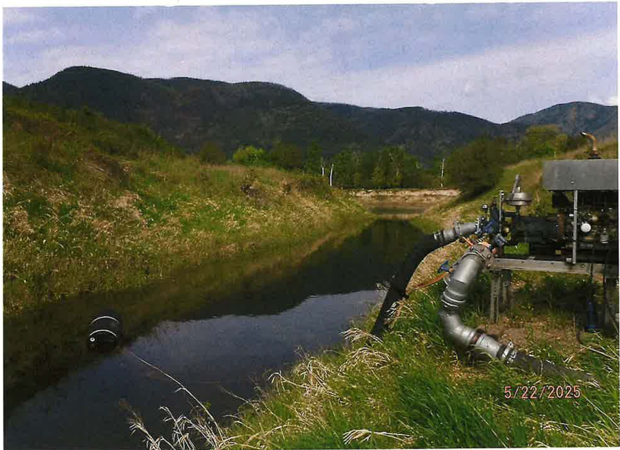
POD – CORNELL PUMP HAS A 3-INCH DISCHARGE ORIFICE THAT IS COUPLED UP TO A 6-INCH SOLID FLEXIBLE RUBBER HOSE
