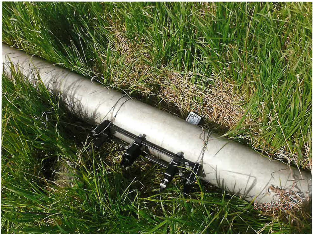
DEPARTMENT GE PT-900 FLOWMETER USED TO TAKE FLOW MEASUREMENTS ON FIRST FULL LENGTH SECTION OF 8-INCH ALUMINUM PIPE
