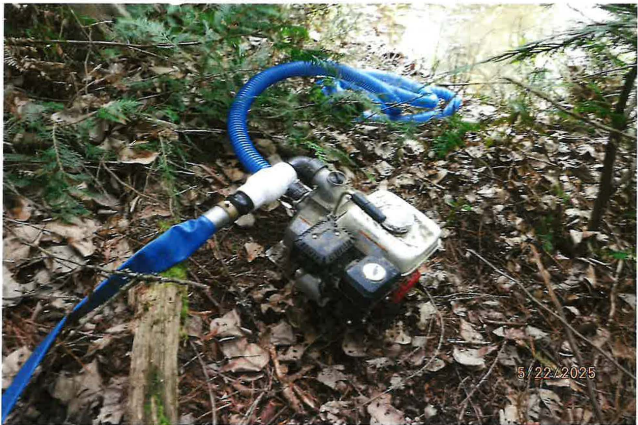
IRRIGATION FROM STORAGE SMALL GENERATOR FRAMED WATER TRANSFER PUMP
