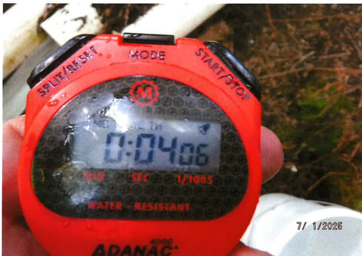
5-GAL BUCKET MEASUREMENT ATTEMPTED AT TIME OF EXAM (LESS THAN 5 SEC FILL TIME)
