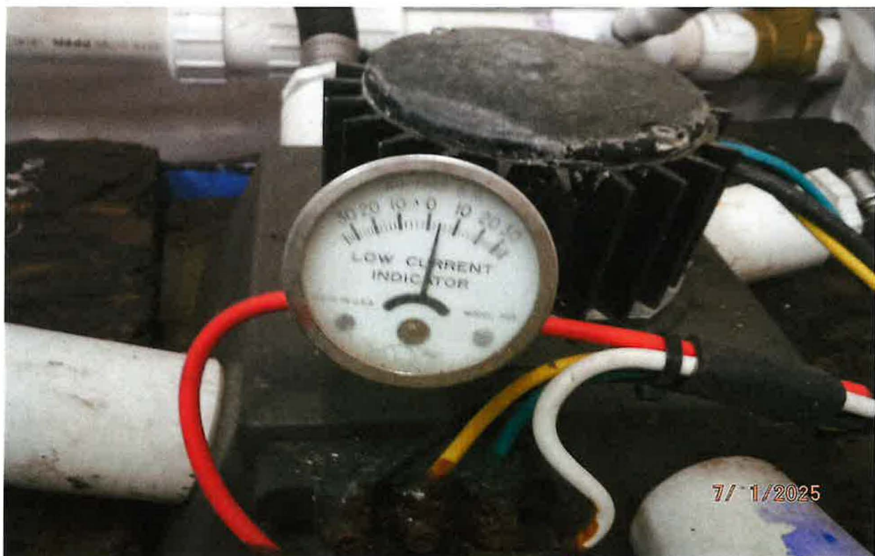
POWER SYSTEM AT TIME OF EXAM MEASURING 4 AMP/HR ON LOW CURRENT INDICATOR ~5 (83)
