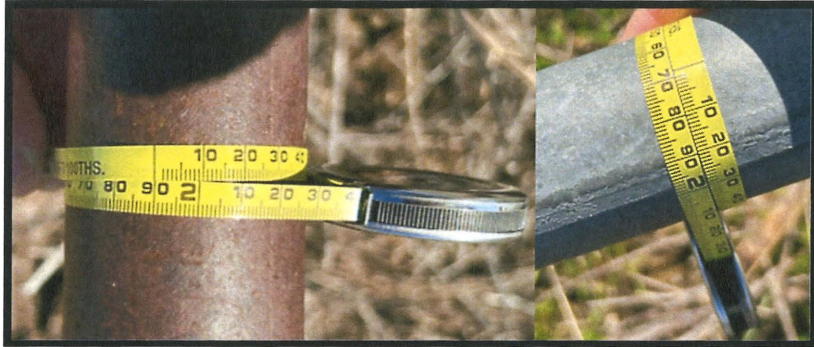
Photos 19 & 20- Diameter measurements for steel mains of cistern well #2 (left image) and cistern well #3 (right image).
