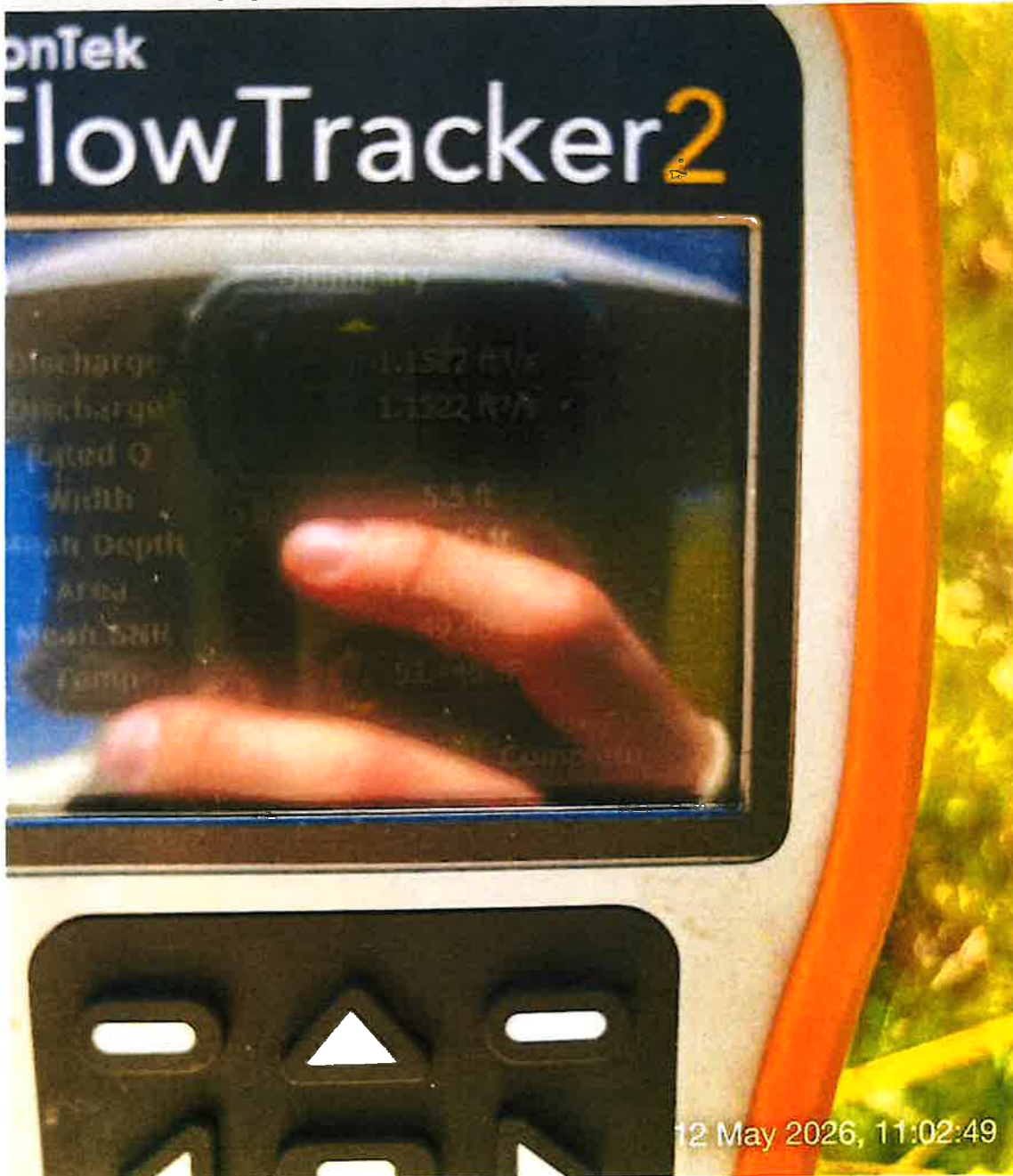
Jensen Ditch flow measurement 1.15 cfs.
