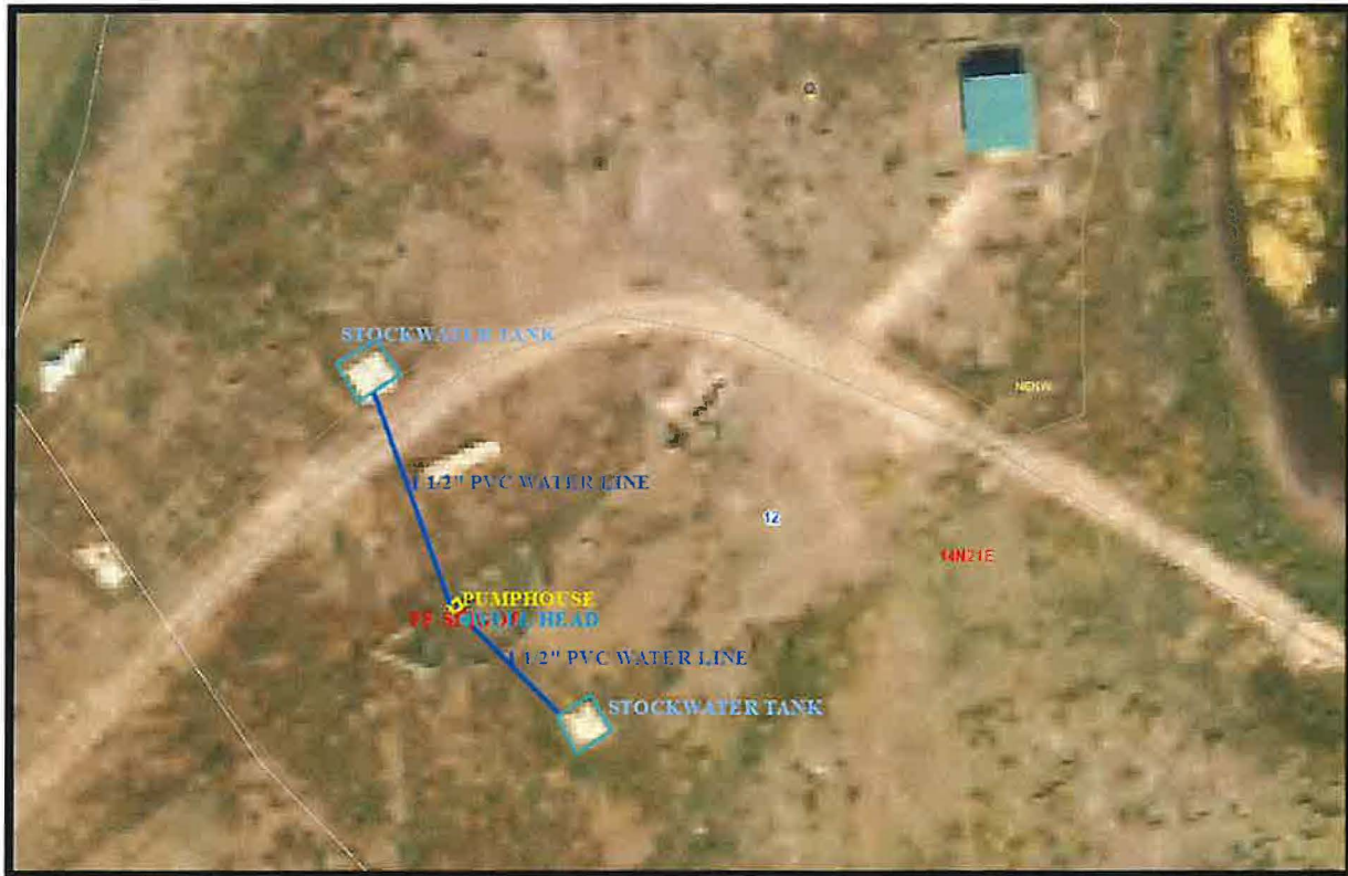
Figure 1- System Diagram – A 2" poly line goes from the well head to the pumphouse. The manifold connects to a manifold with a 44-Gallon pressure tank and an 1 1/2" poly line out to the auto-valve controlled stockwater tanks.
