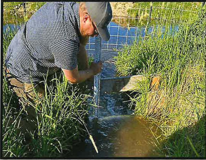
Photos 1 & 2- Left to right respectively. (1) Photo taken from wastewater culvert facing southwest. Cipoletti Weir (2' wide) measurement taken using staff gauge. (2) Photo taken facing northwest from confluence with L-9 Ditch. Weir is installed plumb and level.
