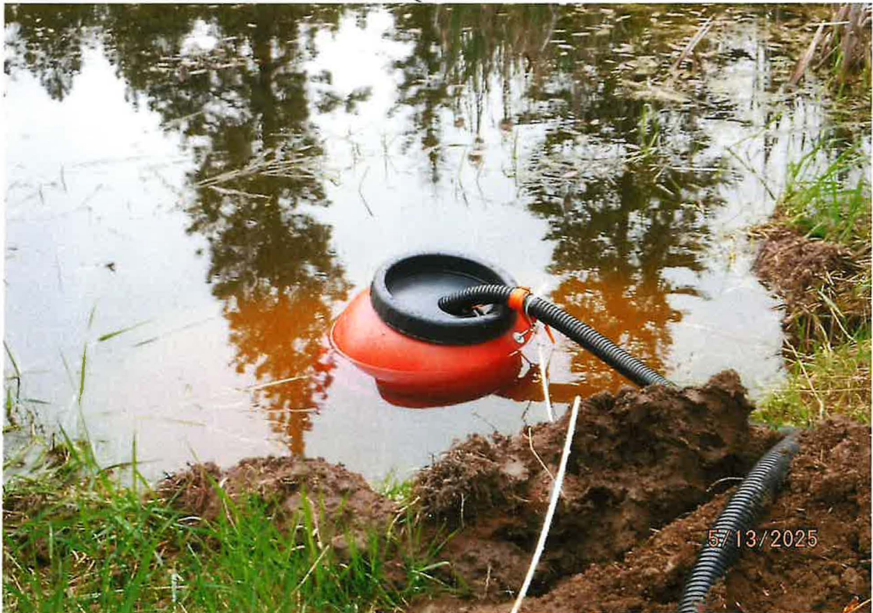
7-HP GENERATOR FRAMED TRANSFER PUMP SET UP ON STANDBY IN THE EVENT FIRE PROTECTION WATER IS REQUIRED TO SUPPRESS AN ACTIVE FIRE
