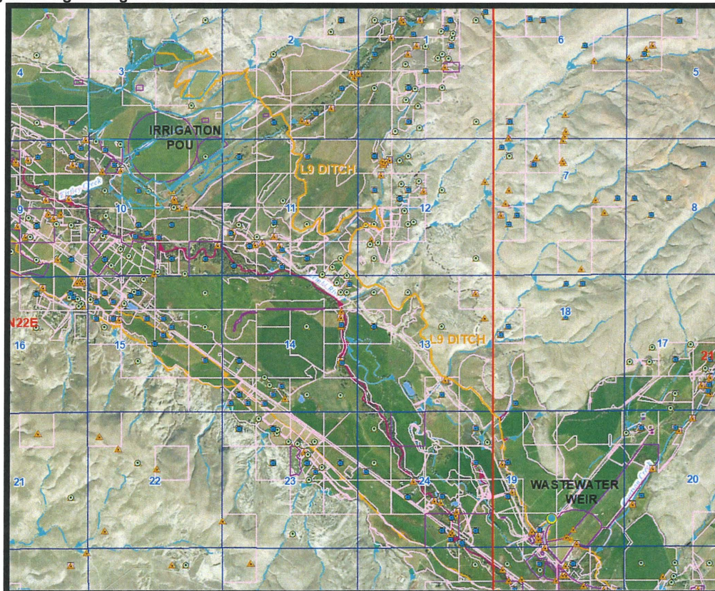
Figure 1b- The L9 ditch sidles the periphery of the valley from the wastewater weir in the southeast to the flood irrigated portions of the permitted POU in the northwest.
