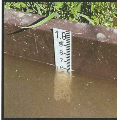
Photos 1-3 – The 12" broad crested weir installed near the southeast corner of the fields along Geertson Creek. In the image on the right the flow crossing the flume can be seen discharging into the L9 Ditch in the background.
