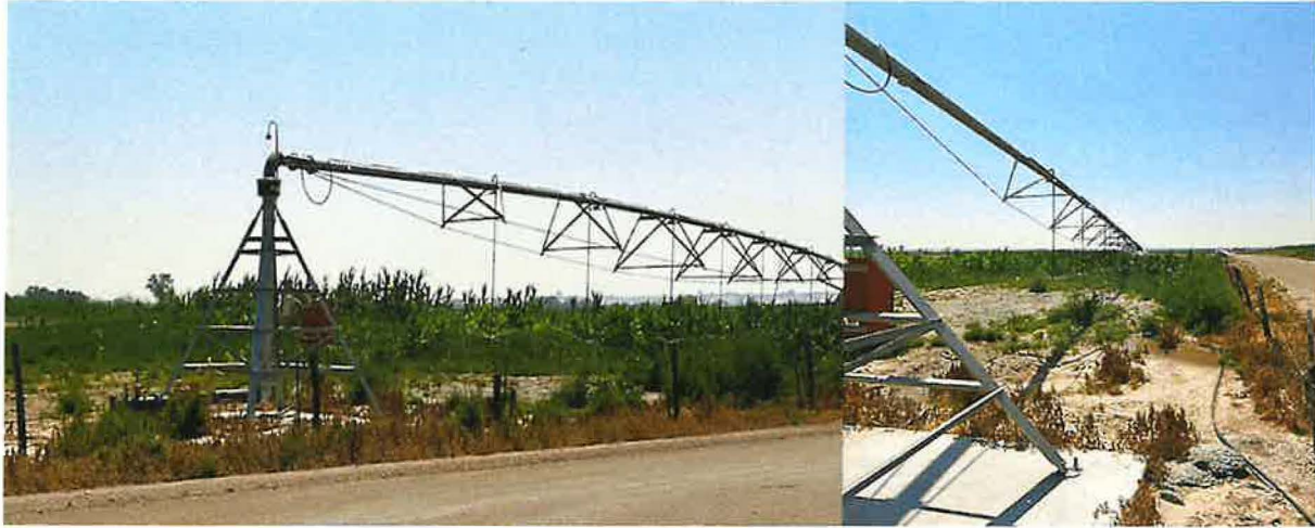
Photo 3- Pivot #2- comprised of 6 spans, each with 6- Nelson Hi-Flo, 20psi-with rotator heads. End guns were visible from the road.
