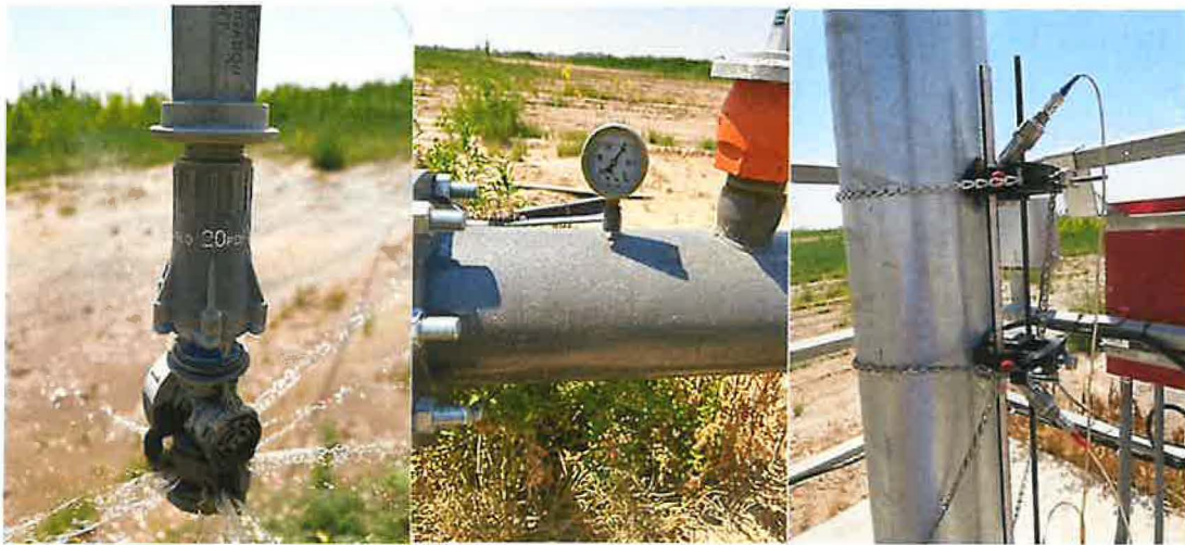
Photos 4-6, From left to right- Nelson Hi-Flo 20psi regulators with rotator heads. Pressure gauge at pivot (reading 40psi). Panametric transducers attached to Pivot #2, while taking measurement.
