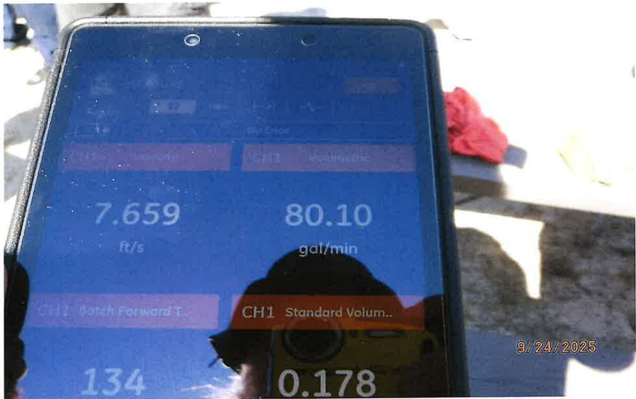
EXAMPLE OF FLOW MEASUREMENT CAPTURED FOR 11 MINUTE TIMED EVENT ILLUSTRATES 80.1 GPM PUMP CAPACITY
