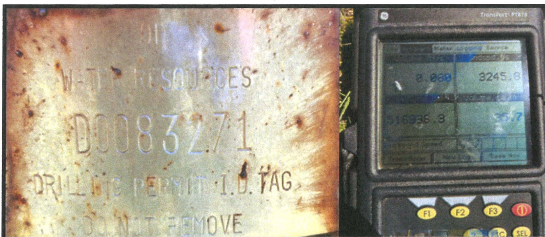
Photos 18 & 19- Irrigation well tag and live reading (0.08cfs) while recording measurements the hand line irrigation system.
