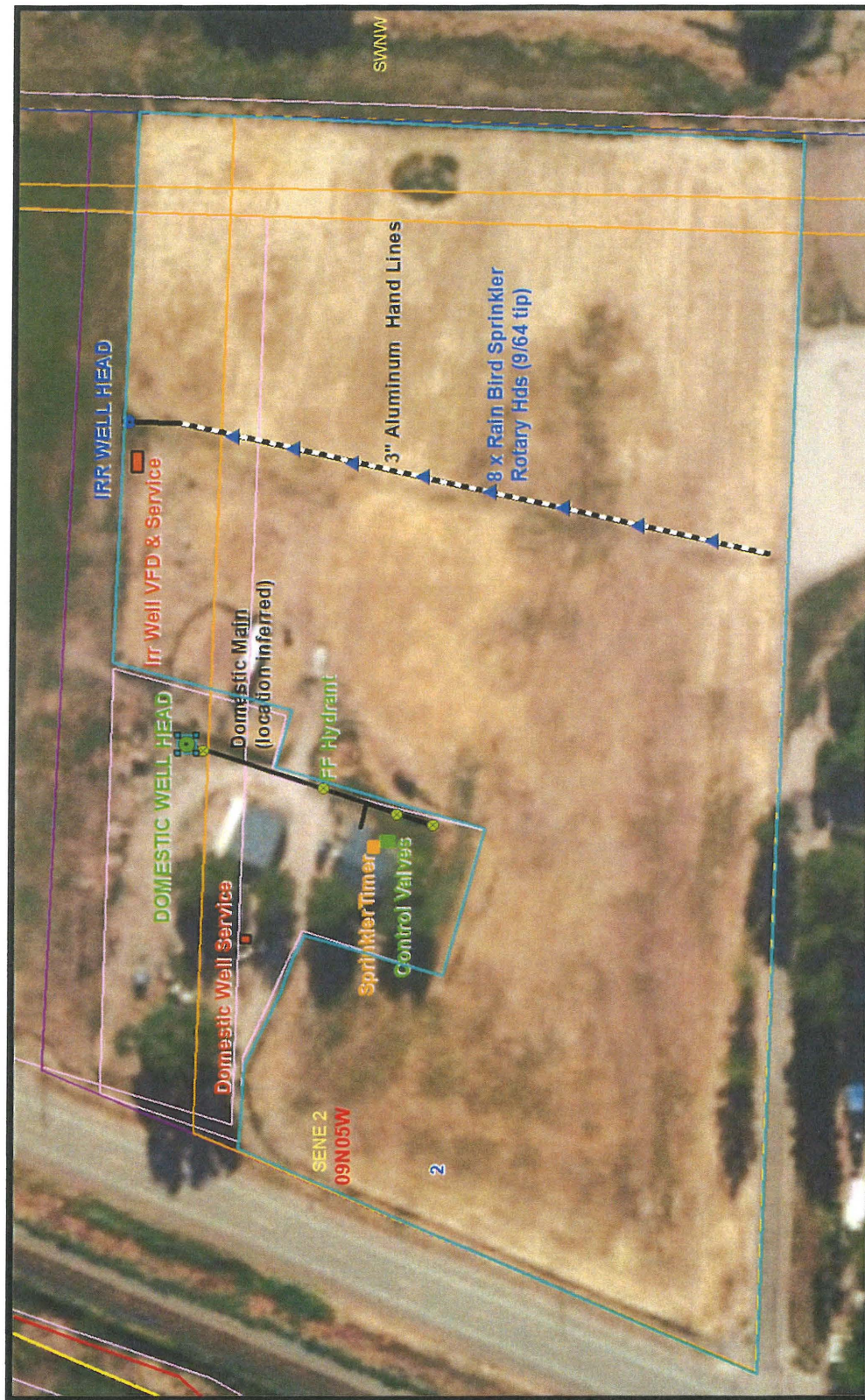
Figure 1- NAIP 2023 imagery- IRRIGATION SYSTEM DIAGRAM. The permit holder had a rack of more than 2 dozen 3"aluminium hand lines which are used in various configurations to irrigate through out the POU. A separate well, pump, and system provide water for domestic uses including in home, less than ½ acre of irrigaton for the lawn, landscape, and garden beds as well as stock watering from frost free hydrants located within the domestic enclosure.
