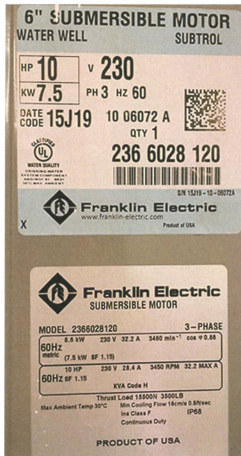
Figure 30 Pump specification tag for D0039476.
