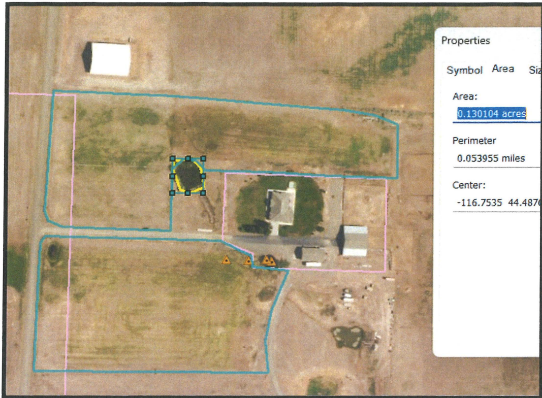
Figure 2- GIS measurement of the pond located west of the home. Areas irrigated using the risers are outlined in blue.
