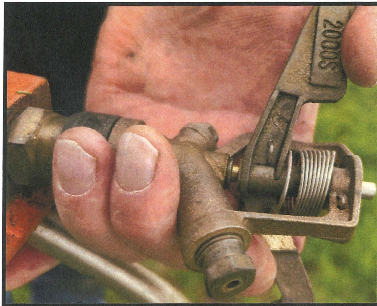
Photo 16- 2000S sprinkler heads with 9/64" tips installed on the wheel lines.
