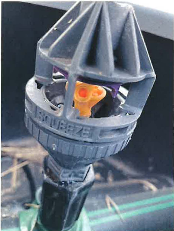
Figure 8. Photograph of K-pod nozzle (#18 Gold R33LP at 50 psi= 4.1 gpm per nozzle).
