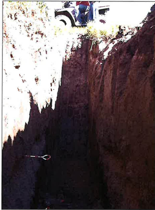
Figure 18. Backhoe pit showing maximum depth at approximately 7.5 feet (Soil Pit 2).
