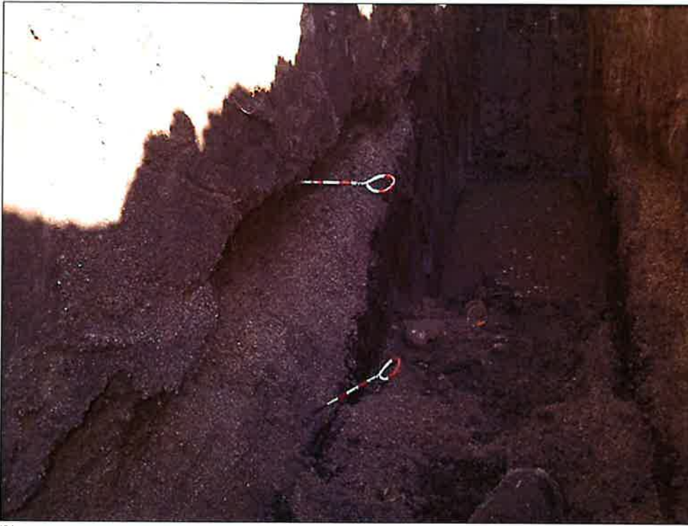
Figure 22. Wall of Soil Pit 2 showing non-cohesive, sand channel overlying peat.
