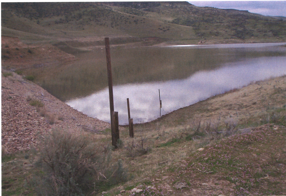
Figure 4 Staff gages used to measure active reservoir level.
