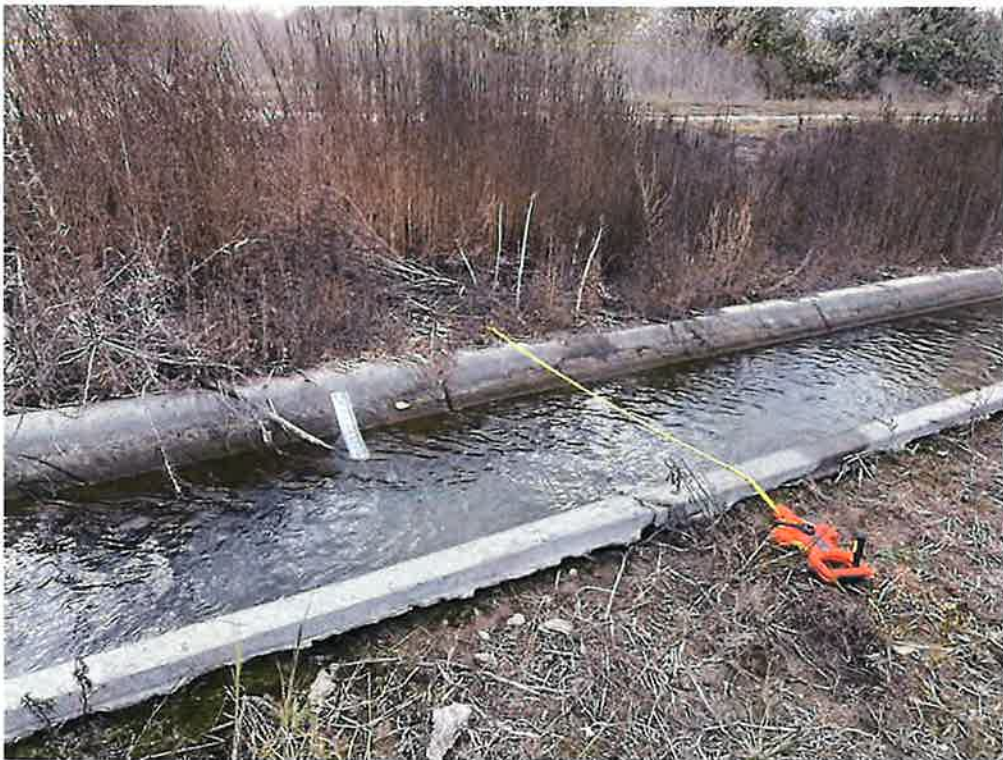
Flow measurement in West Ditch below bifurcation.
