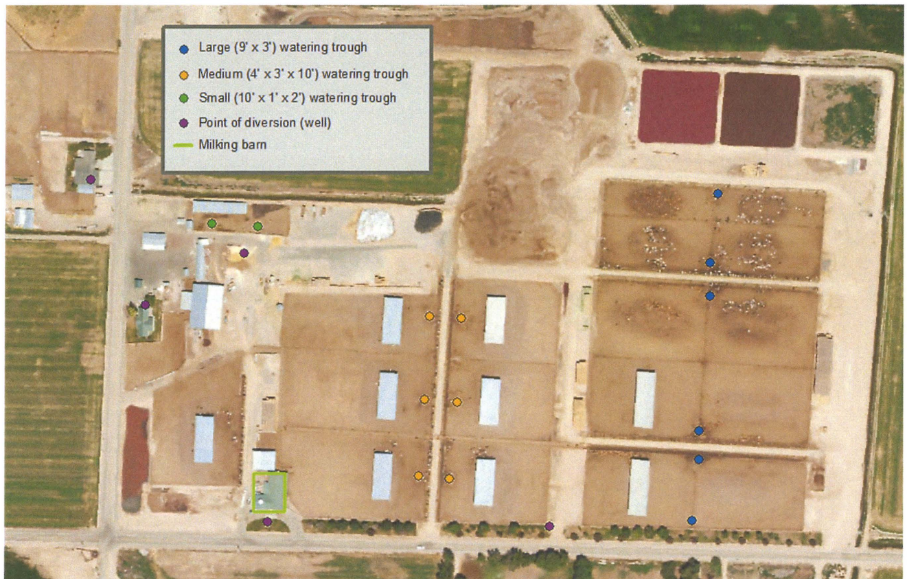
Figure 2 System diagram includes all stockwater locations and points of diversion. Mainlines from wells to stock tanks are not included since the actual locations and routes are unknown.
