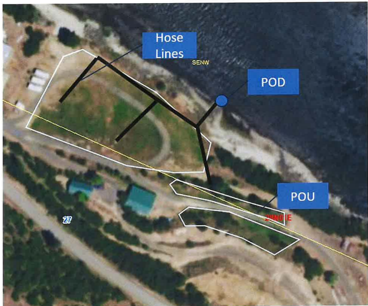
Figure 1: Permit Diagram. Only 2 of 3 hose lines are used at once.
