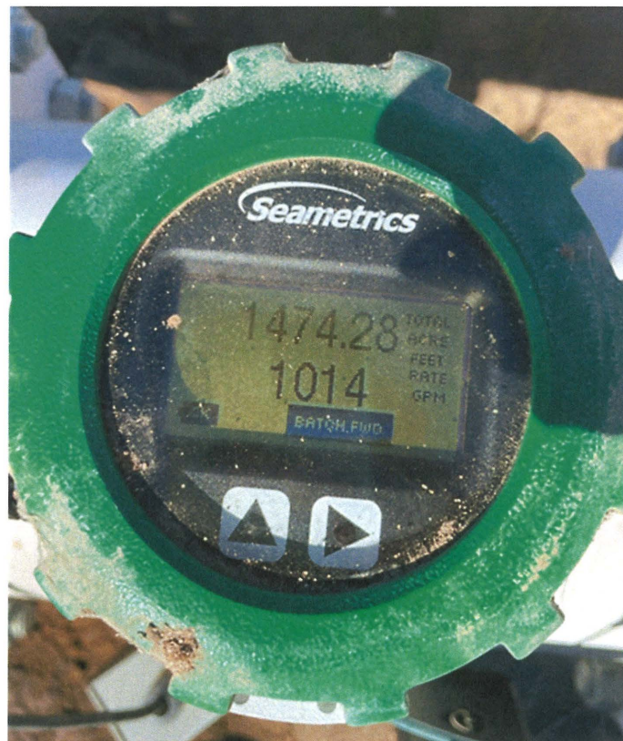
Figure 17 Seametrics agriculture flow meter on well 306583 showing an output of 1014 gallons per minute.
