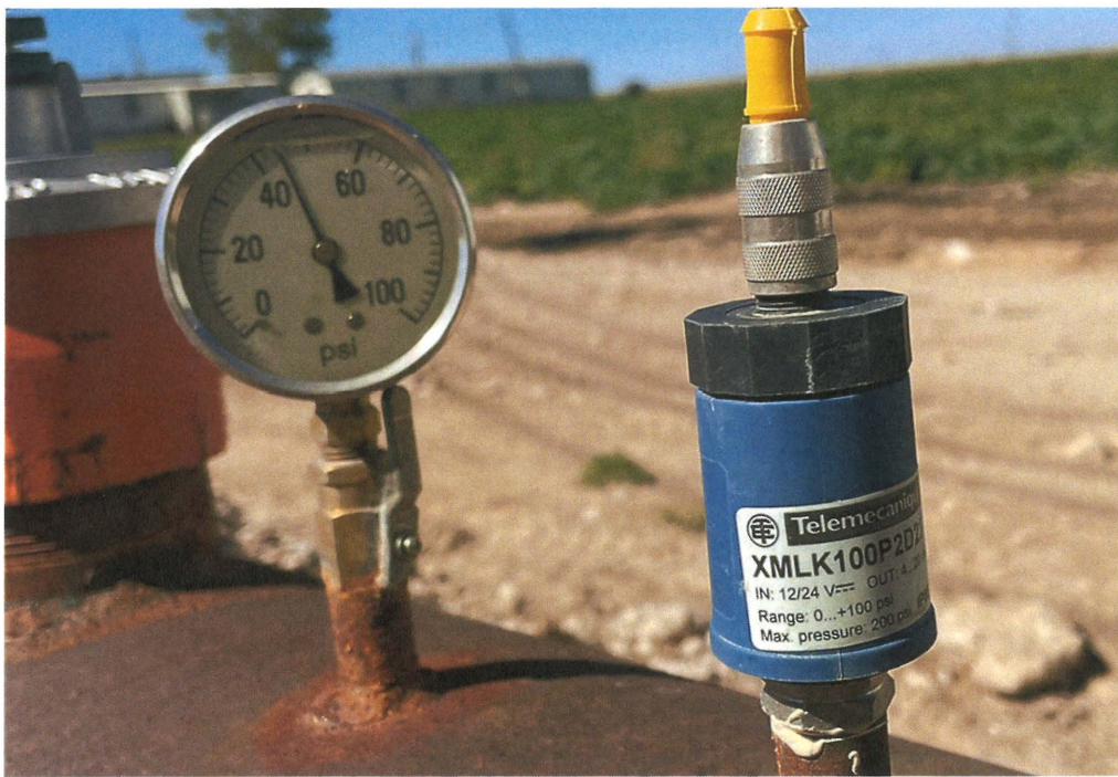
Figure 8 Pressure gage for well D0057945 reading 45 PSI, also reflected on the digital monitor screen in figure 5.
