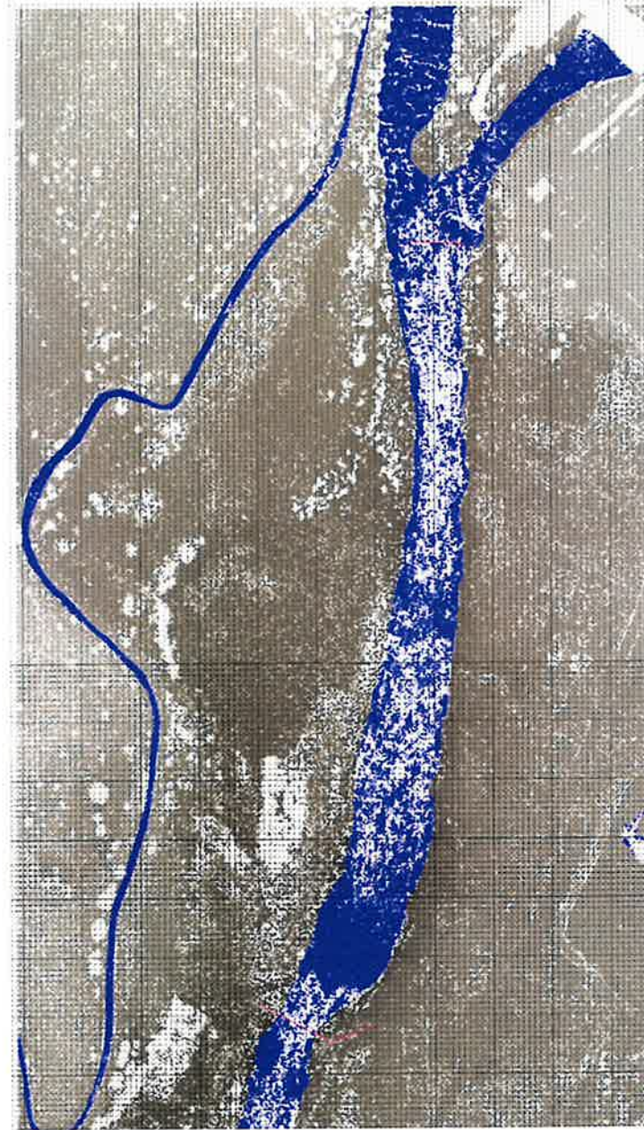
Figure A.1 Classified lidar point cloud (only ground and water classified points used) with grid lines used to identify the upper end of the reservoir and the dam (shown in thin red lines) when overlaid on the September 2004 Google Earth image. Solid grid lines are shown every 100 feet with dashed grid lines every 10 feet.
