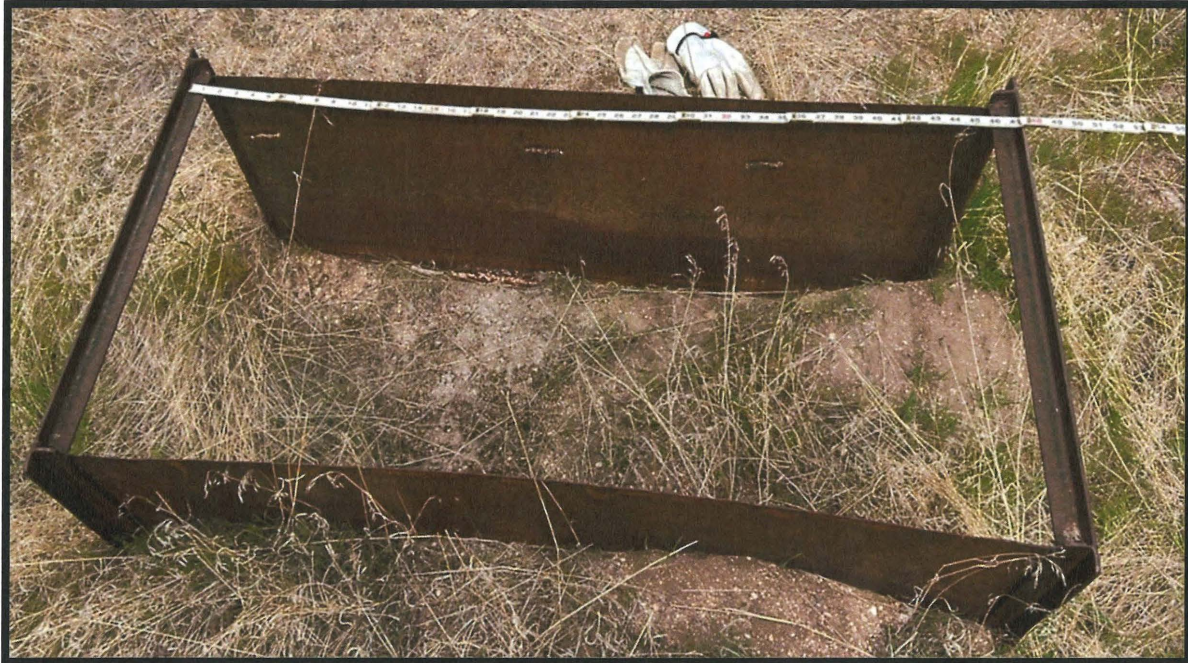
Photo 11- Weir length measurement (48" total length). North is up in the image.
