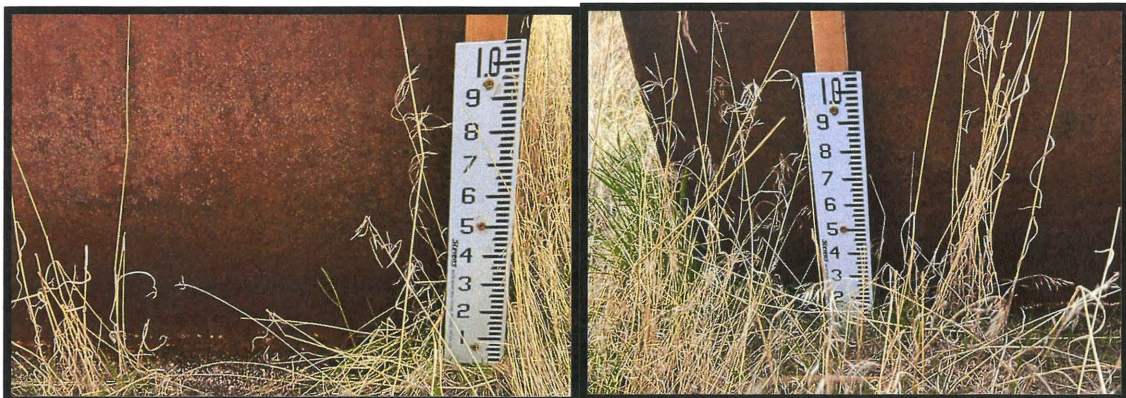
Photos 14 & 15- Staff gauge measurements taken at the west (downstream) end of the weir.
