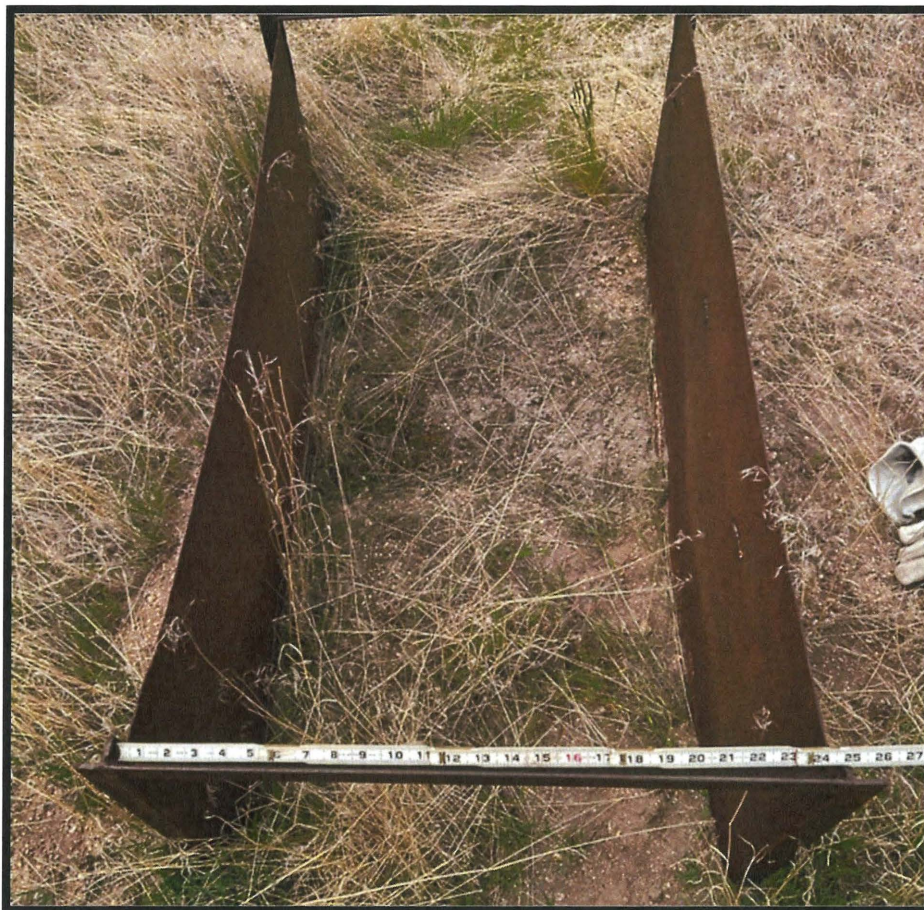
Photo 10- Weir diameter measurement (24" wide).
