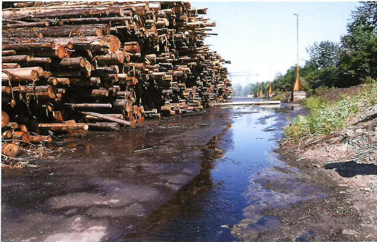
INDUSTRIAL FROM STORAGE POU – LOG WATER EXCESS CHANNELIZES BACK TO SETTLING PONDS FOR RE-CIRCULATION PROCESSES (REDUCES TOTAL DIVERSION VOLUME FROM WATER SOURCE THROUGHOUT SEASON)
