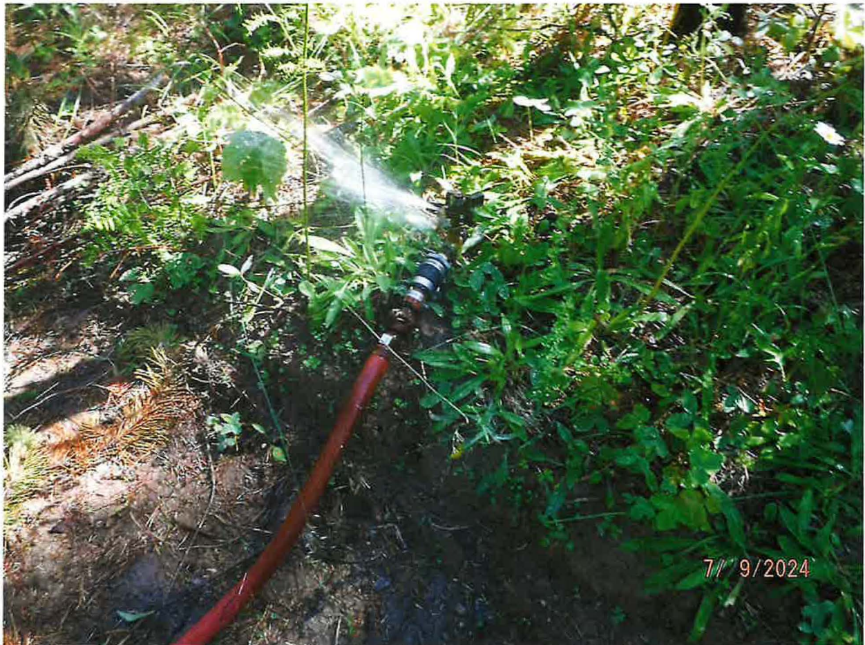
1-1/2 INCH FIRE HOSE COVENYANCE TO SPRINKLER SYSTEM, WHICH IS REDUCED DOWN TO A 3/4-INCH BRASS IMPACT SPRINKLER
