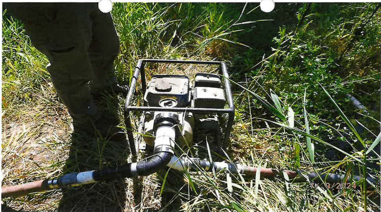
POD – UPPER 24-HR IMPOUNDMENT POOL; POWER MAX XP650WP, GENERATOR FRAME 6.5 HP PUMP
