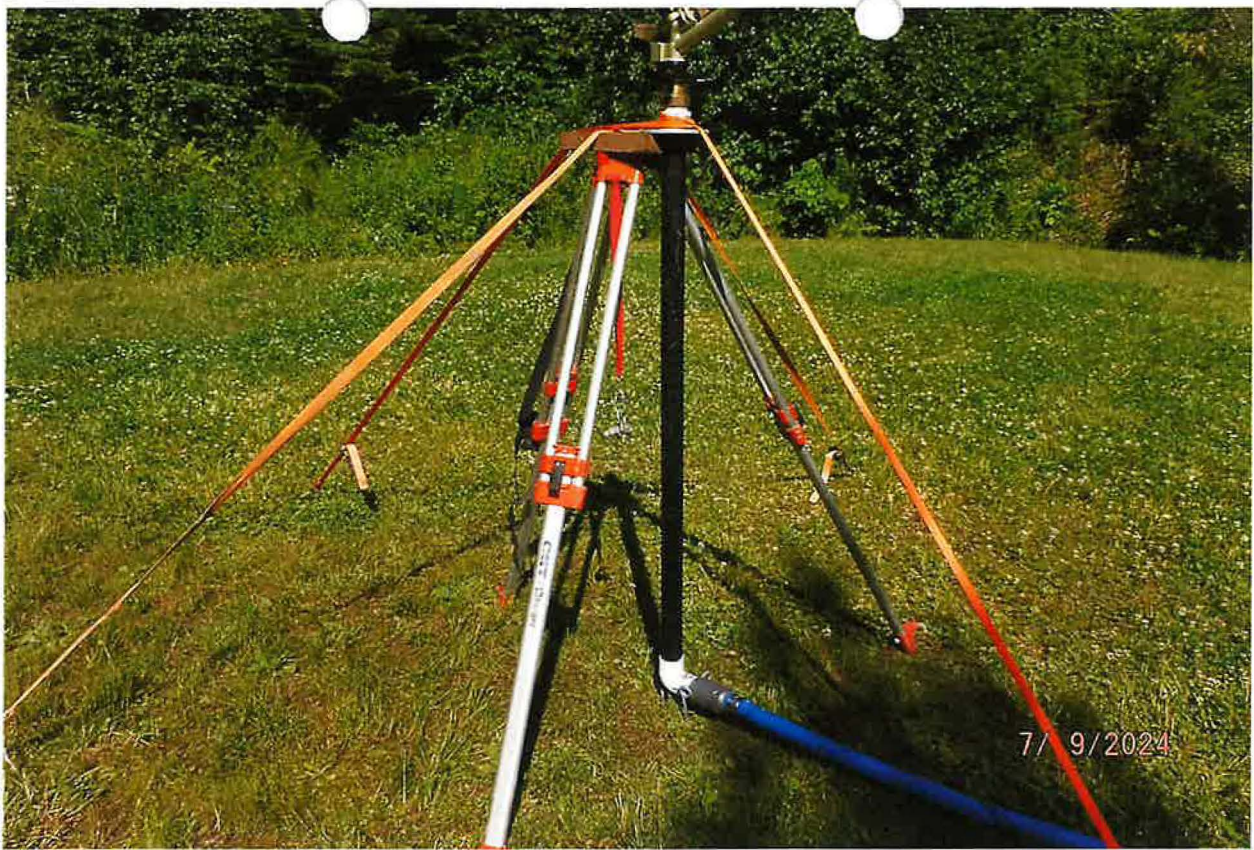
BIG GUN SPRINKLER PAIRED WITH NORTHSTAR WATER TRANSFER PUMP & FIRE HOSE(S)
