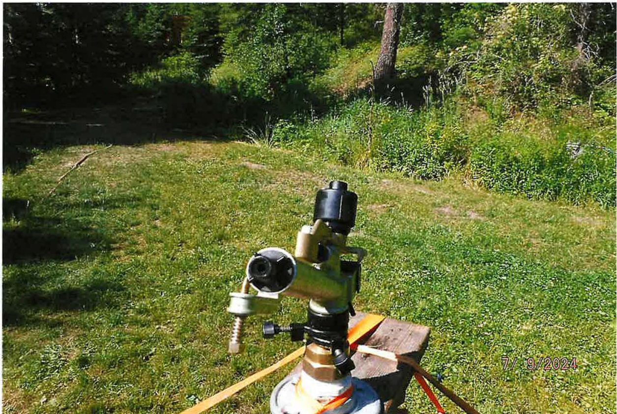
BIG GUN WITH 8MM NOZZLE WITH 1-1/2 INCH STANDARD PIPE THREAD
