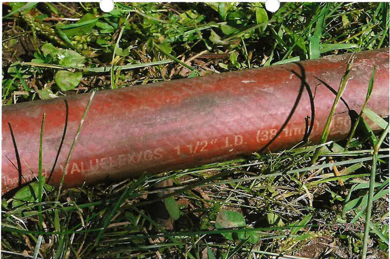
1-1/2 INCH FIRE HOSE COVENYANCE TO SPRINKLER SYSTEM, WHICH IS REDUCED DOWN TO A 3/4-INCH BRASS IMPACT SPRINKLER
