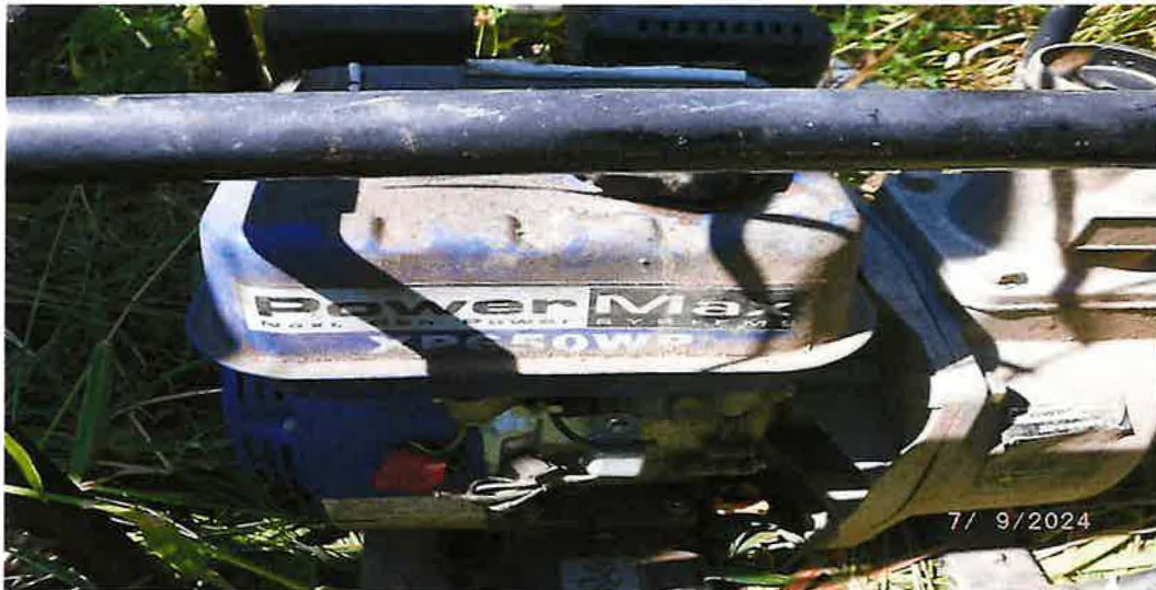
POD – UPPER 24-HR IMPOUNDMENT POOL; POWER MAX XP650WP, GENERATOR FRAME 6.5 HP PUMP
