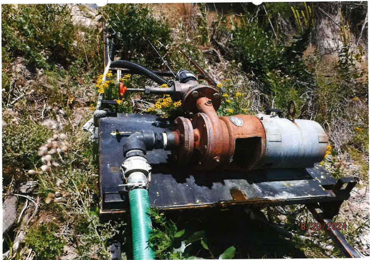
POD – BERKELEY CENTRIFUGAL PUMP WITH 2-INCH DISCHARGE PORT
