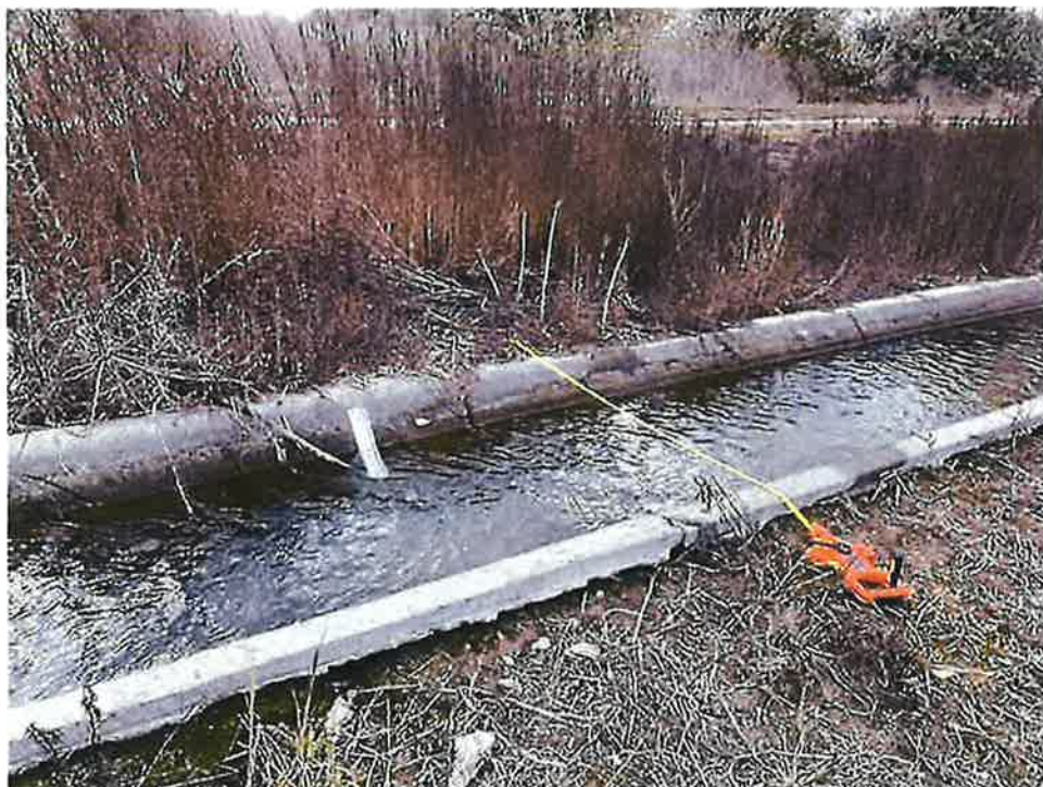
Flow measurement in West Ditch below bifurcation.
