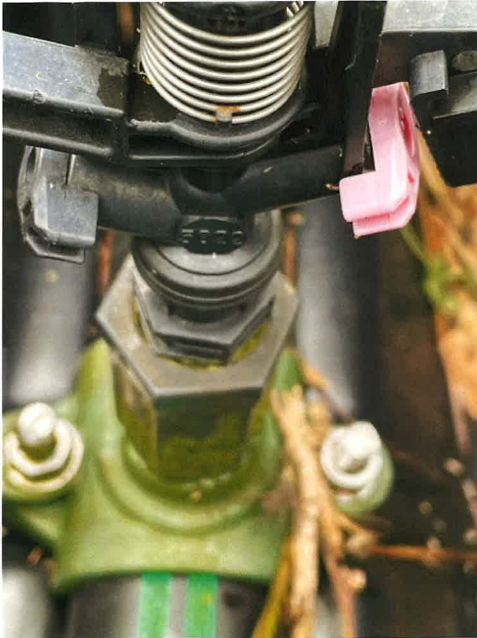
Figure 7: KLine 5022 Sprinkler with 3.00 mm nozzle
