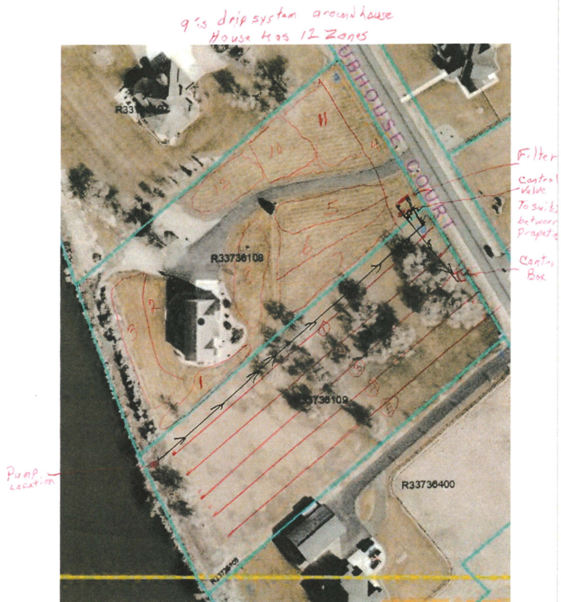
Figure 1 System diagram provided by the permit holder to represent the irrigation zones, pump location, and control box.
