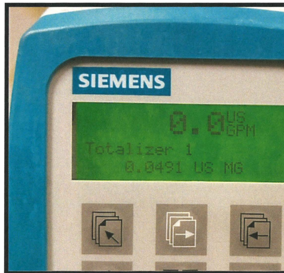
Photo 6- Potable totalizer reading taken at the start of the field examination was 0.0491 mil gallons=94,100 gallons=0.2 AF.
