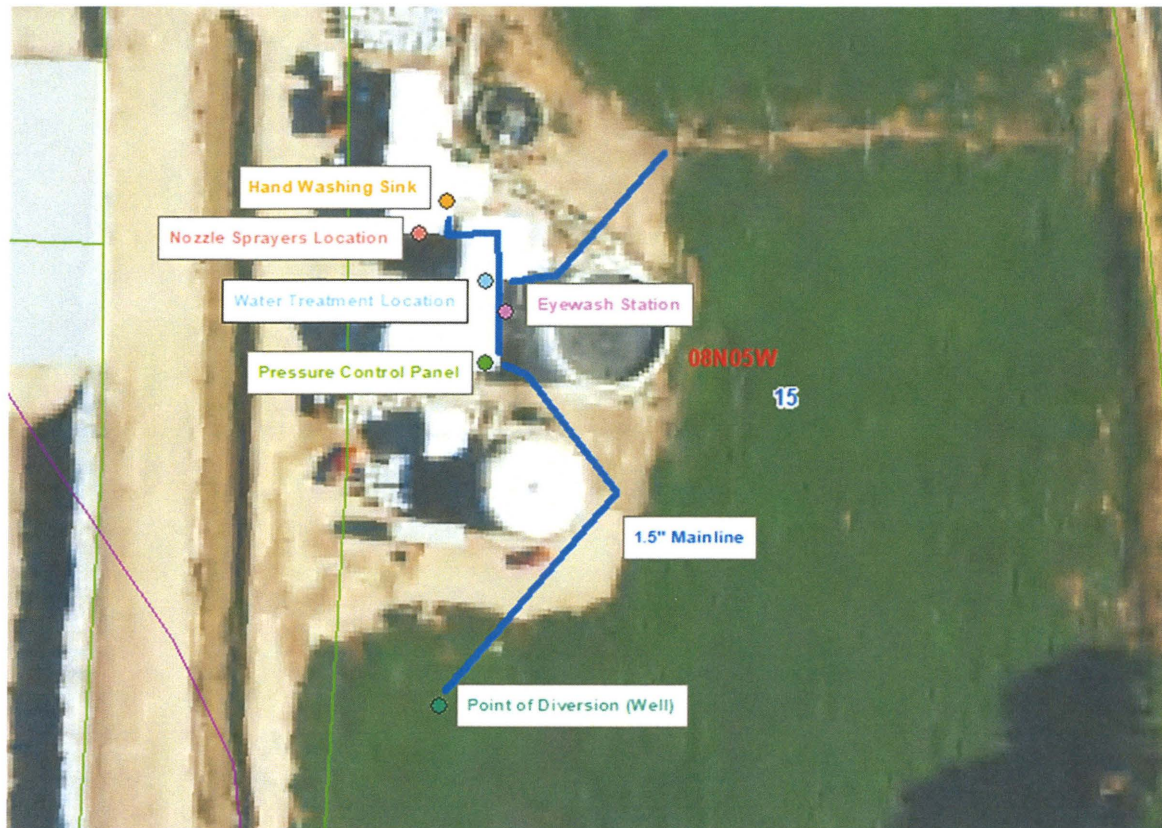
Figure 2 System diagram showing route of fresh and waste water to all amenities under WR 65-24209.
