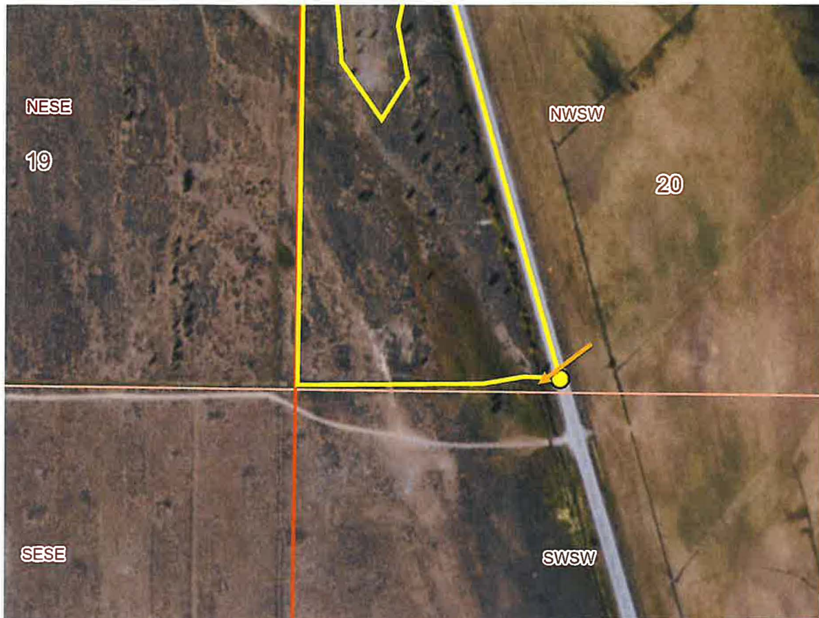
Figure 3. The orange arrow indicates the location to be plugged at the head of the lateral ditch running west from the unnamed drain.
