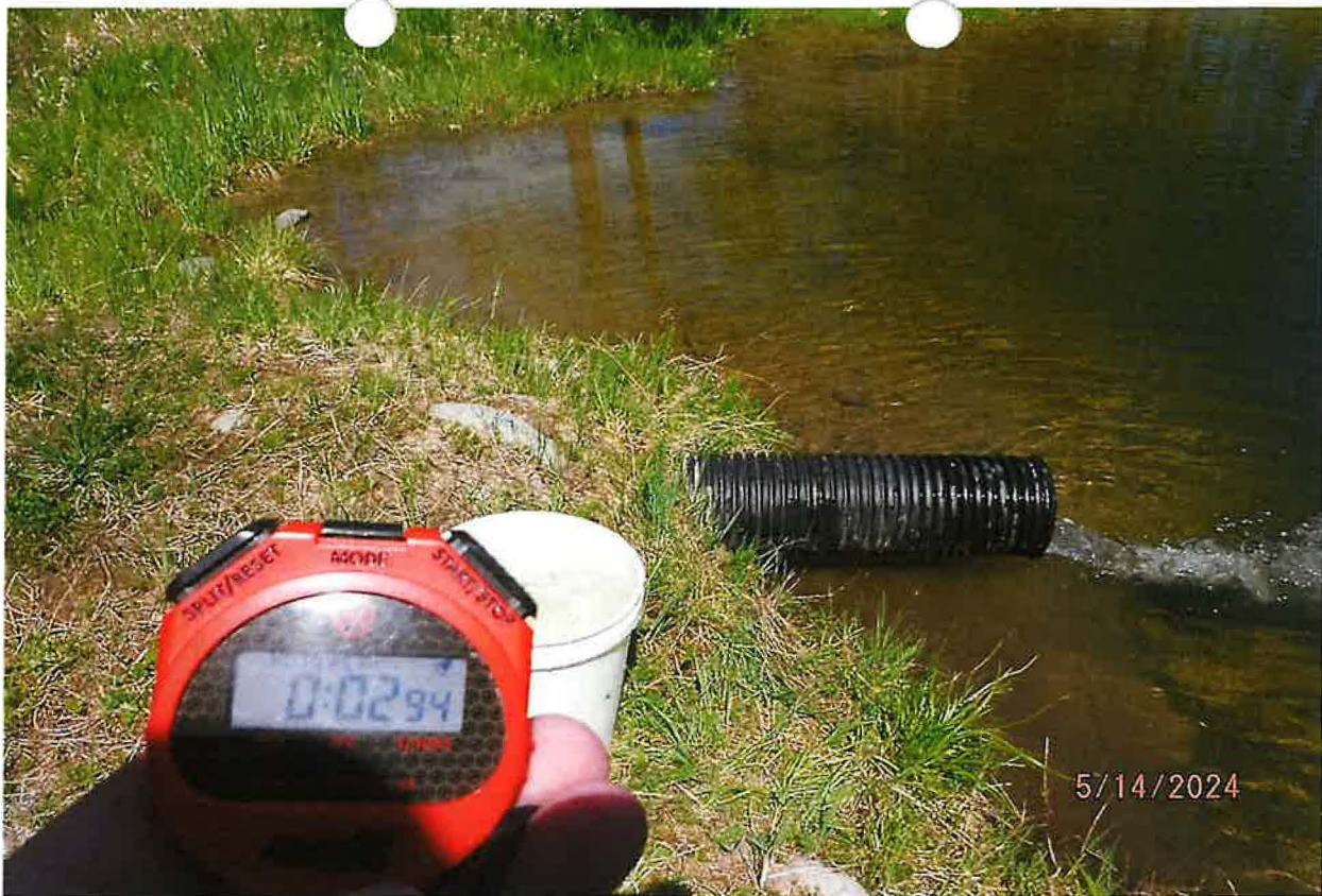
RECREATION (FLOW THROUGH WATER) POU – INFLOW TO POND FROM CONVEYANCE DITCH & PIPE CIRCULATES WATER WHICH OVERFLOWS BY EARTHEN CHANNEL TO LOWER GRADE POND(S)
