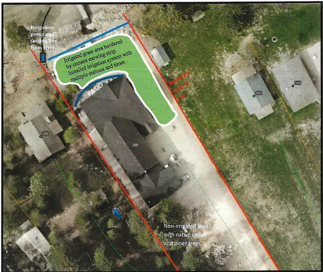
Figure 3- Diagram of irrigated POU and POD outlined with details including system type and non-irrigated areas.
