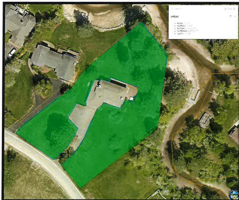
Figure 3- Bonner County GIS imagery- Both Irrigated POU measurements areas are stacked and shaded in highlighted boundary is the top layer. Approximately 1.2 acres of irrigated area determined using an ArcGIS measurement and measurements made with the Bonner County imagery using a map submitted by the permit holder as a reference.
