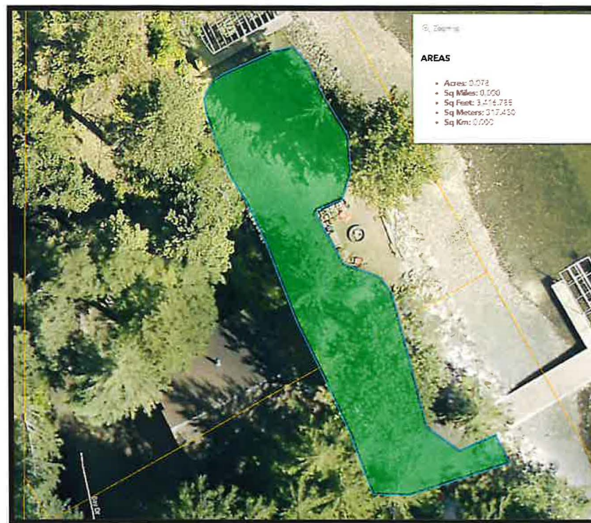
Figure 3-Bonner County GIS-imagery measurement of the irrigation POU described by the permit holder. The area along the rip rap at the shore has a paver path from the wet dock to the dry dock, and there is no irrigation further west than the paver path from the house to the dry dock.
